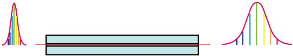
Figure 3.3: The light of longer wavelength travels slightly faster and spreads the pulse out[1]
