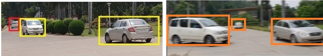
(a) Cars detected with yellow represent their detection from networks trained with F_{Gauss}, F_{Edges}, F_{Opt} and conv5_{F_{Int}} whereas car detected with black represents their detection from networks trained with F_{Gauss}, F_{Edges} and F_{Opt} only (b) Cars detected with orange represent their detection from networks trained with F_{Gauss} and F_{Opt}
