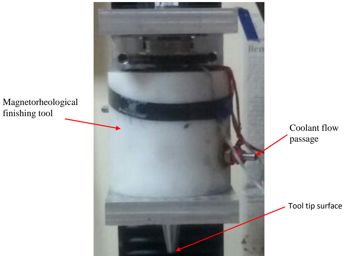
Figure 3.2 Photograph of ball end magnetorheological finishing tool to measure the tool tip surface temperature.
