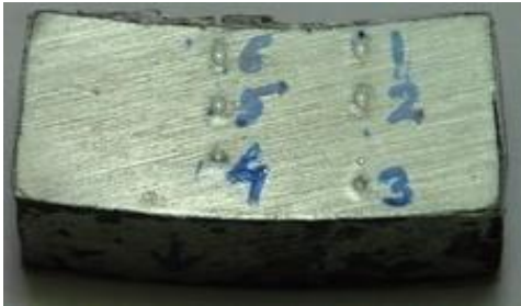
Fig. 4.11: SS 304 Specimen at 0% CW Level
