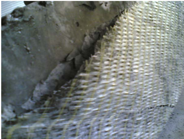
Plate 6.4 Debonding of GFRP Jacketing with Fibres at 45 Degree to the Longitudinal Axis of Beam
