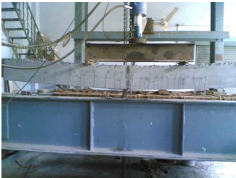
3U90(1)- at Failure
