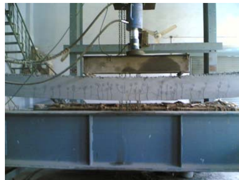
3U75(2) – at Failure
