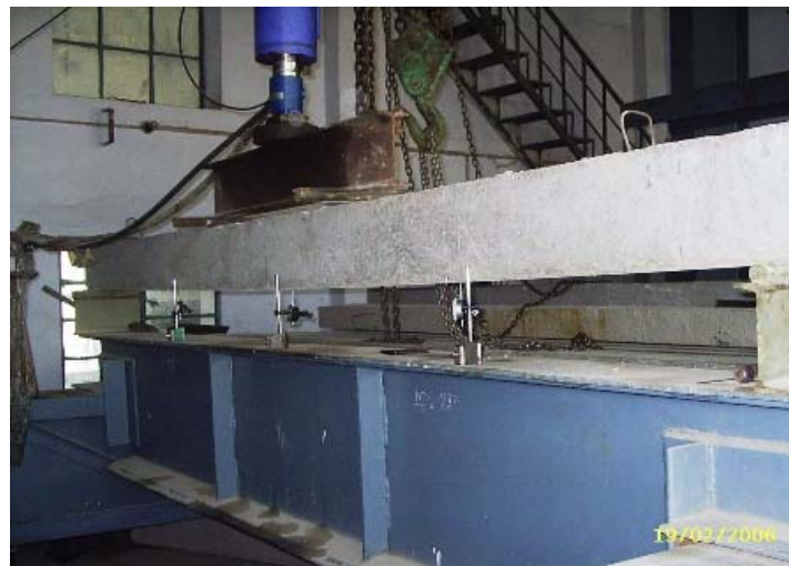
Plate 3.3 Test Set up for simply Supported Beams Subjected to Two-Point Loading with Dial Gages at Mid-Span and Quarter Span Section
