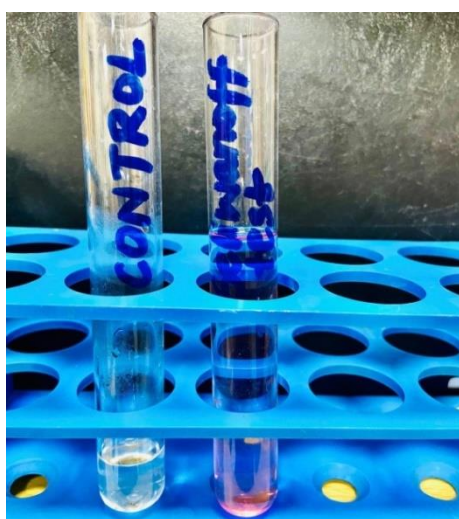
Figure 4.10: The above figure represents colour change in test tube containing levansucrase from transparent to cherry red due to presence of fructose.
