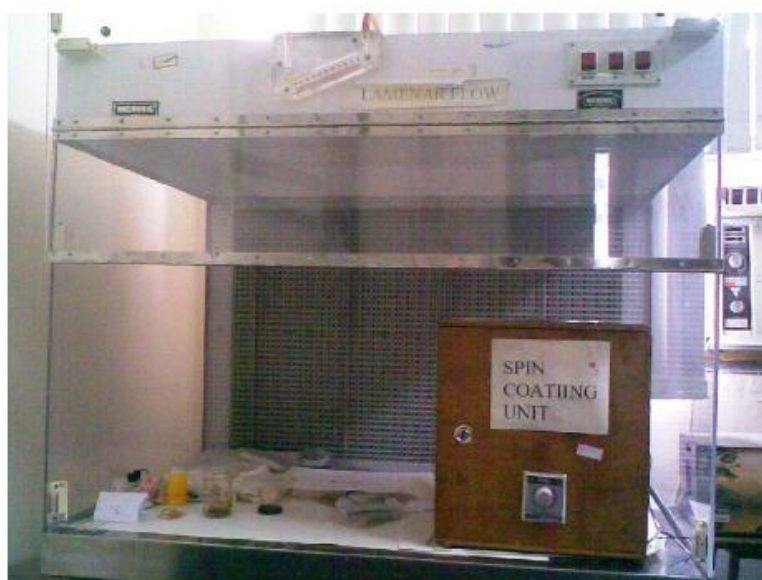
Figure 3.2: Spin coating unit for depositing thin PVDF composite films
