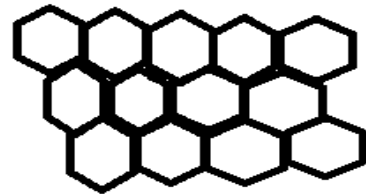
Fig.7.2 Hexagonal close packing
