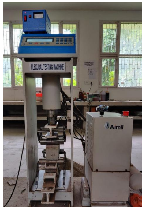
Figure 3.12 Flexural testing machine with arrangement of concrete prism in between supporting and loading rollers
