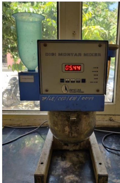
Figure 3.8 Hobart-type laboratory mixer to prepare fly ash amended cementitious grout
