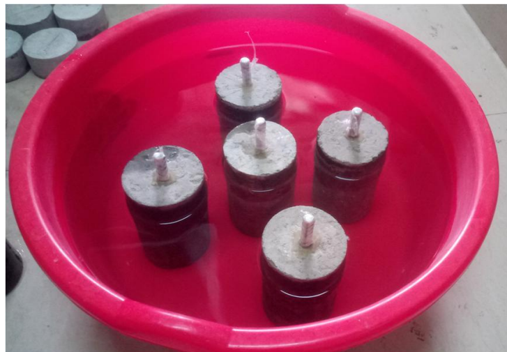
Figure 3.6 Reinforced cylinders exposed to 5% NaCl solution
