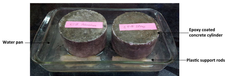
Fig. 1. Arrangement of the sorptivity test.
