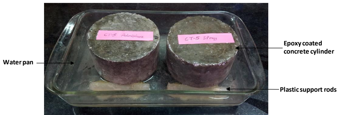
Figure 3.4 Arrangement of the sorptivity test
