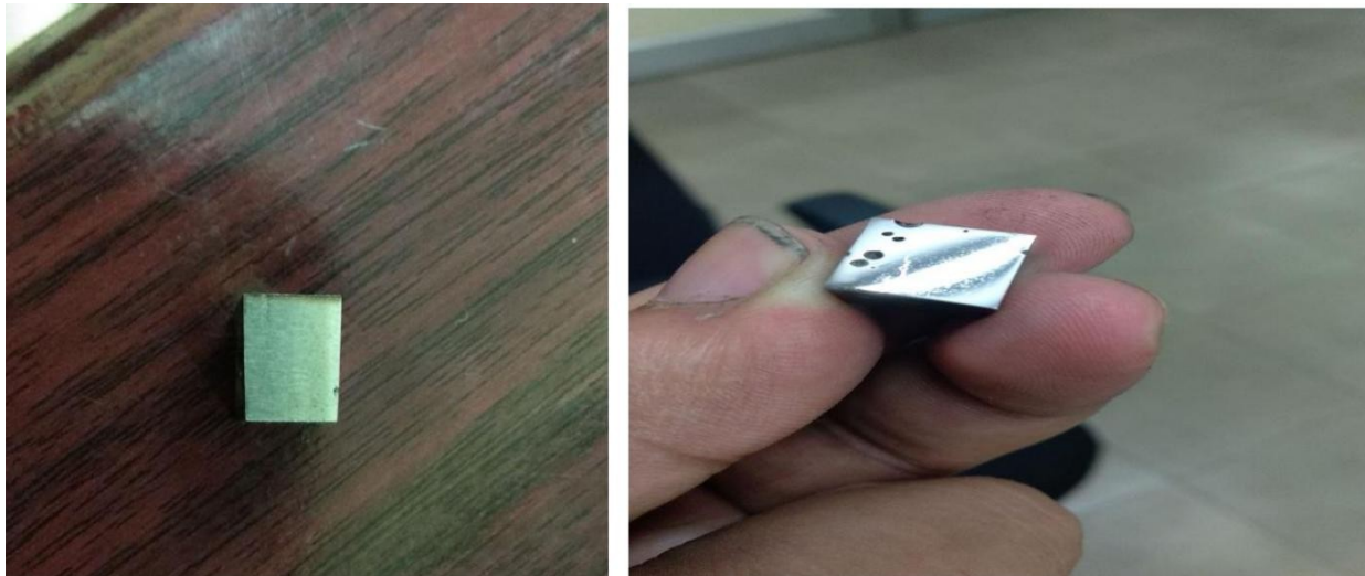
Fig 3.10 (a) Without polishing (b) With Polishing (Courtesy IIT Bombay, Metallurgical engineering & Material science lab)
