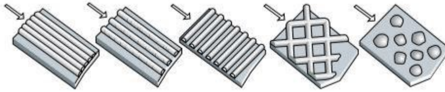
Fig. 1.5 (a) Continuous overlap (b) Regular interval (c) Grid passes (d) Spot welds
