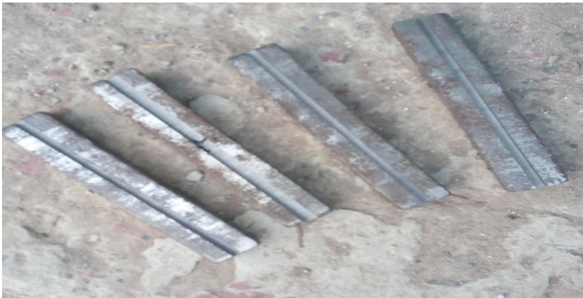
Fig 3.4 Grooving done on cast iron plates (Courtesy TIET workshop)
