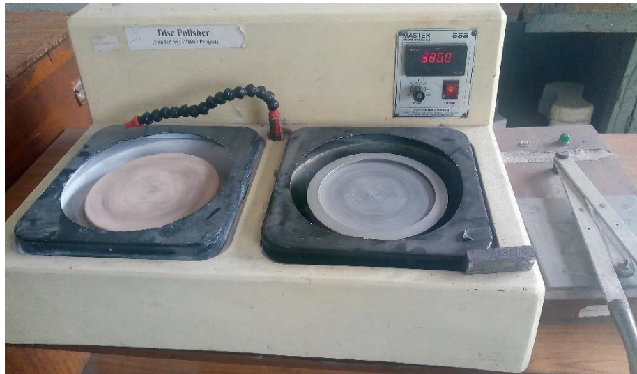
Fig.3.6 Disc Polisher (Courtesy TIET machine tool lab)
