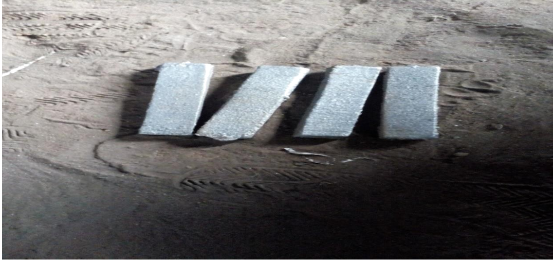
Fig 3.3 C.I. plates after casting (Courtesy R S Industries)
