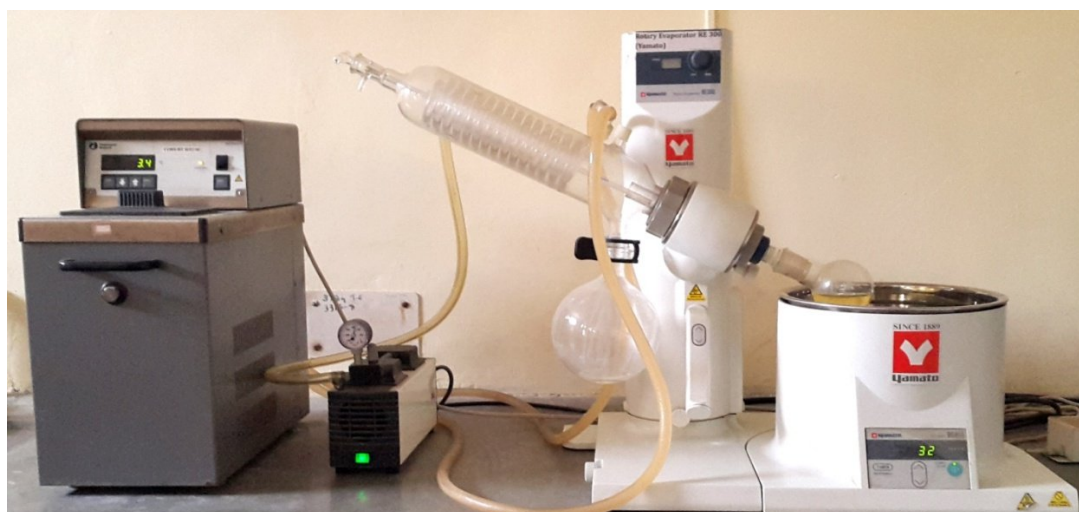
Figure 6: Rotary evaporator during operation
