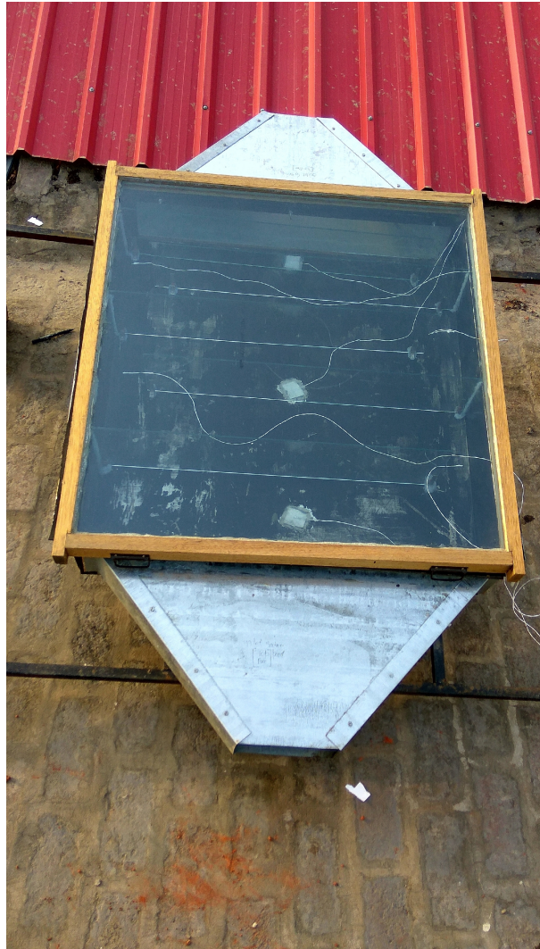
Fig 4.1: Solar air heater with multi-pass adjustment.
