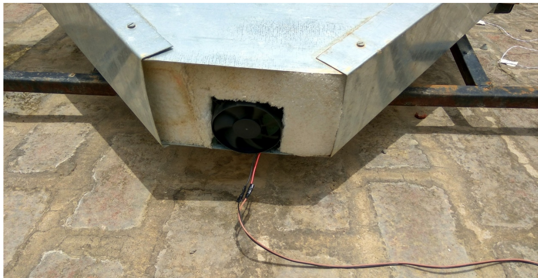
Fig 4.9: Variable speed fan for controlling air mass flow inside solar air heater.
