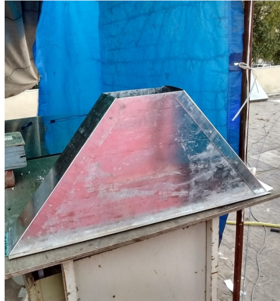
Fig 4.4: Inlet cover of the solar air heater.
