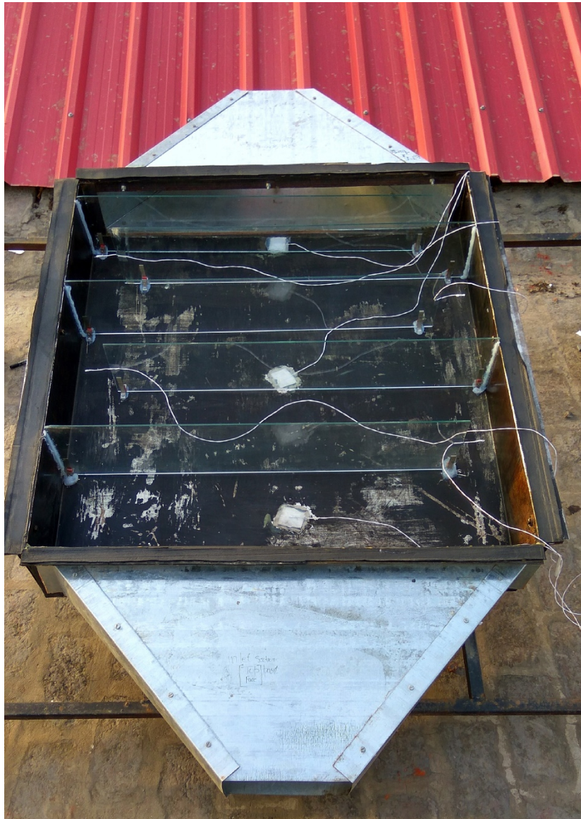
Fig 4.10: Multi-Pass arrangement on absorber plate.
