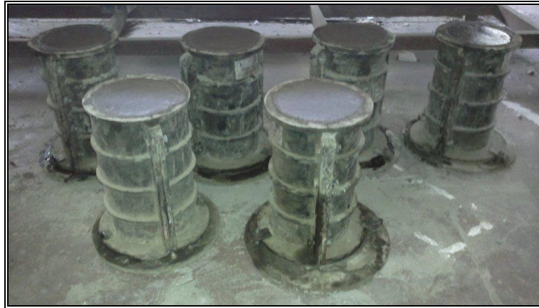
Fig. 3.6 Casting of Cylindrical blocks
