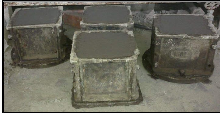
Fig. 3.4 Casting of Cubical blocks
