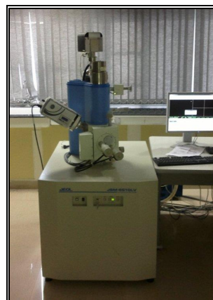
Fig. 3.2 Scanning Electron Microscope (SEM)
