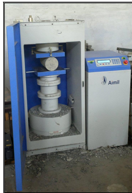
Fig. 3.8 Testing of split tensile strength
