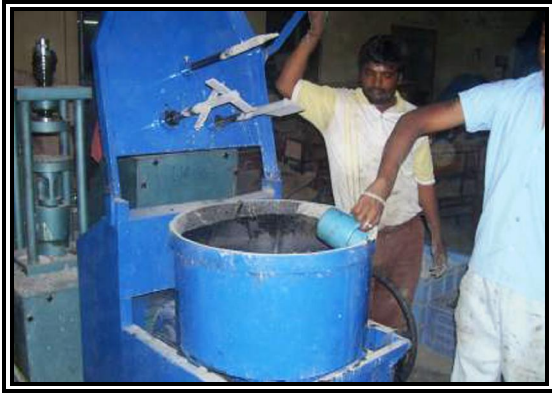
Fig. 2.2 Mixing of slag
