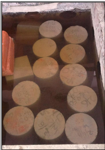
Fig.3.7 Curing of blocks in water tank
