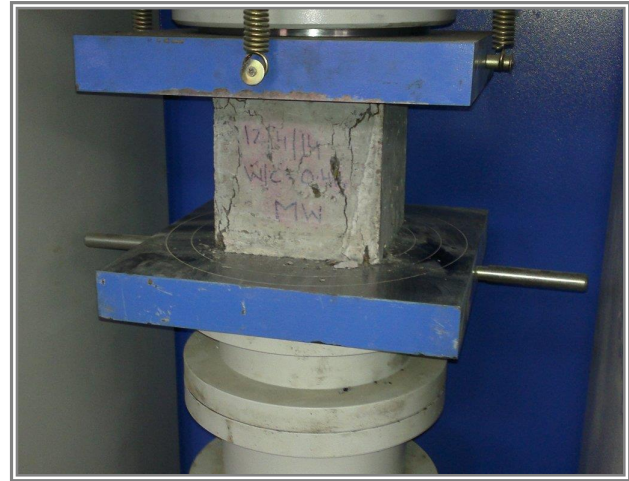
Fig. 3.5 Testing of compressive strength
