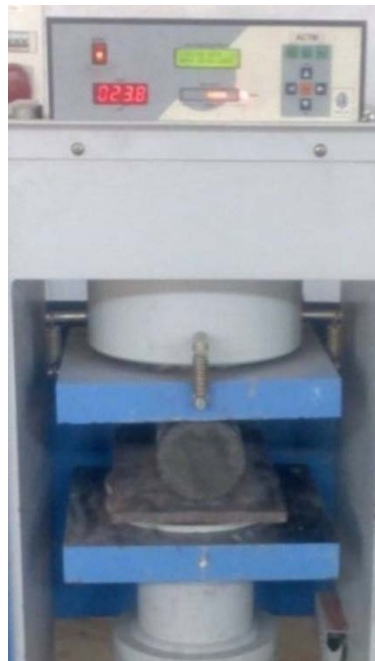
Fig. 4.8: Split tensile strength in progress
