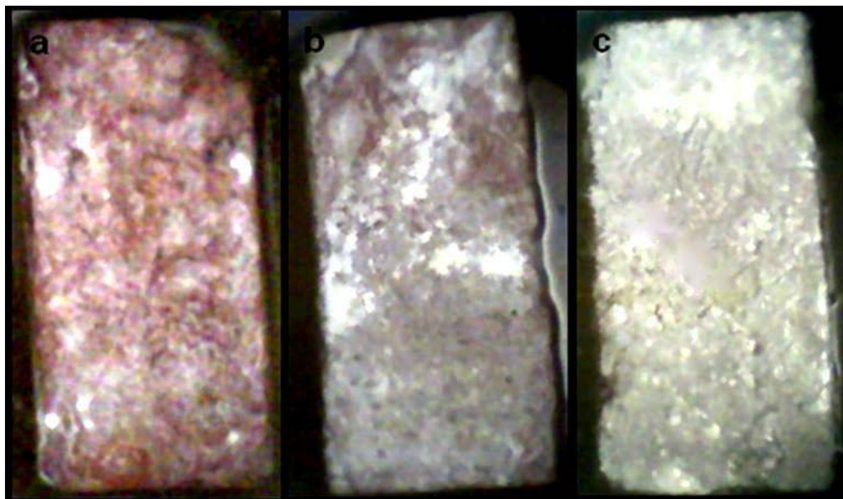
Figure 6.13 Microbial induced calcite deposition on bricks. (a) Control, (b) MICP by S. pasteurii (Bp W) and (c) MICP by Bacillus sp. (CT-5)
