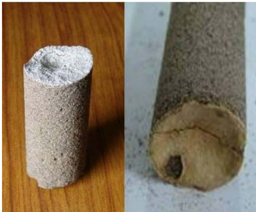
Figure 4.14 Microbial sand plug formed by the bacteria
