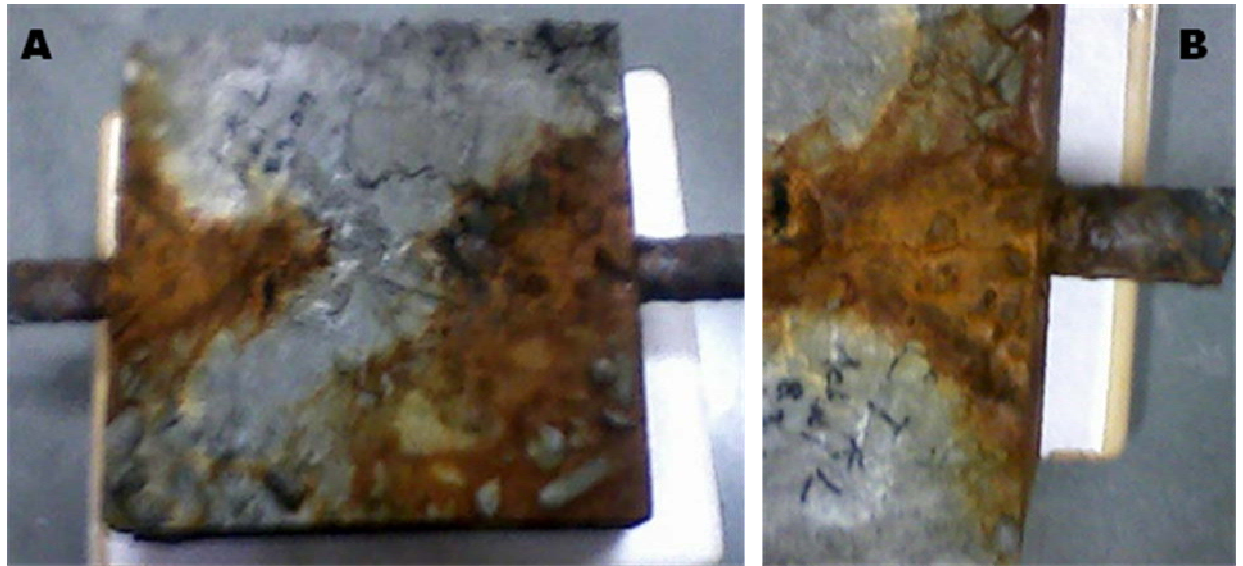
Figure 6.17 (A) RC specimen after corrosion and (B) Visible cracks and red and brown stains of rust on its surface
