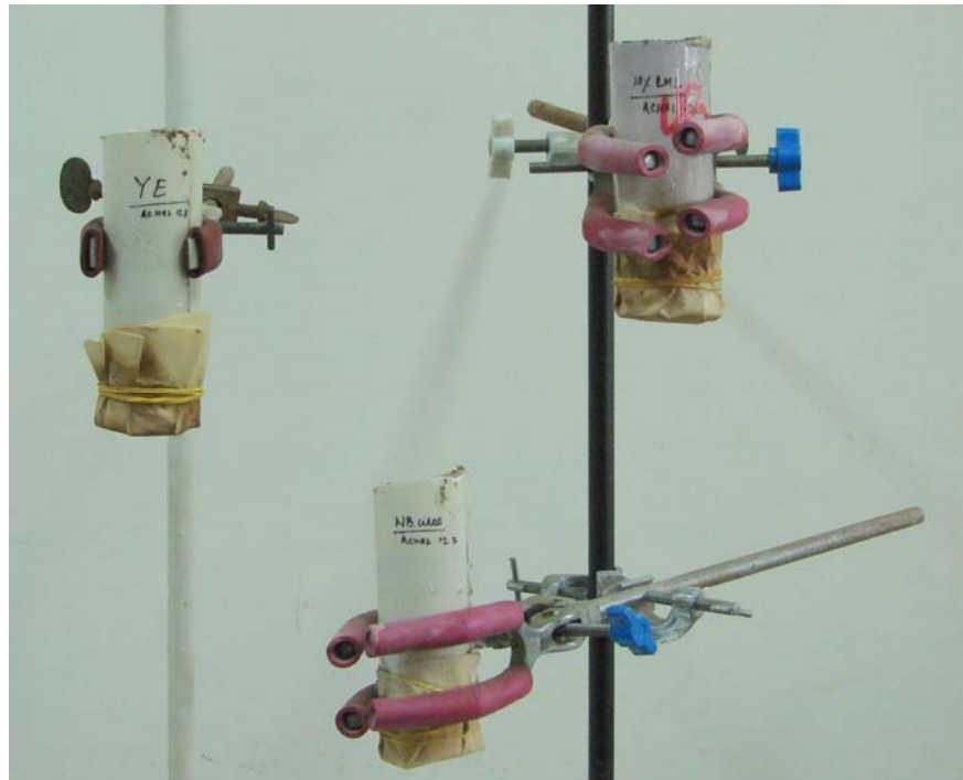
Figure 4.13 Assembly of microbial sand plugging column
