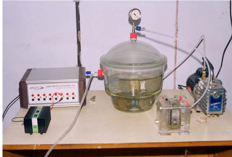
Figure 3.2 Typical set up of RCP test as per ASTM 1202-05 used in this study
