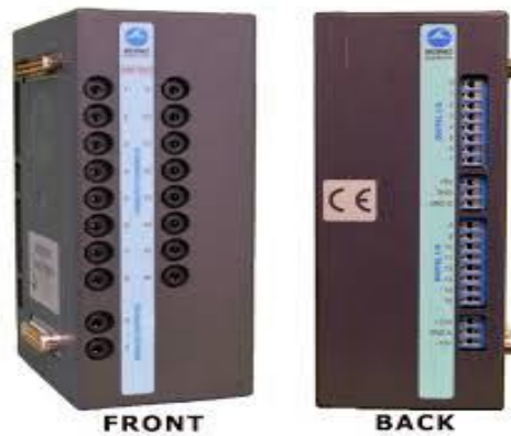
Figure 6.6: Isolated Power Supply Module
