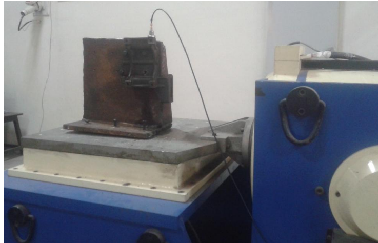
Figure 5.9: Experimental setup for original bracket without compressor
