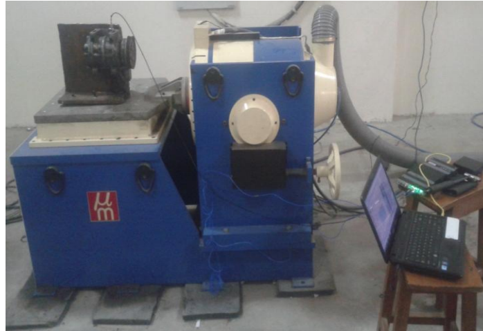
Figure 5.17: Experimental setup for optimized bracket with compressor
