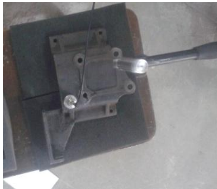
Figure 5.7: Experimental setup during free-free condition of original bracket
