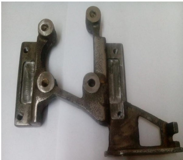
Figure 5.3: Optimized bracket after machining
