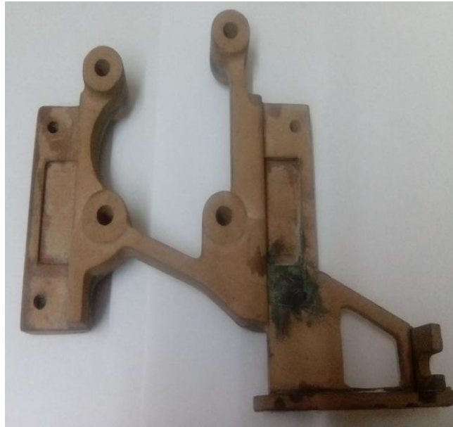
Figure 5.1: Pattern for optimized bracket
