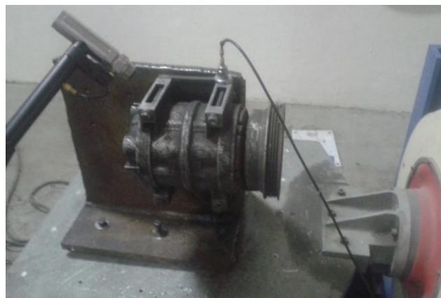
Figure 5.11: Experimental setup for original bracket with compressor
