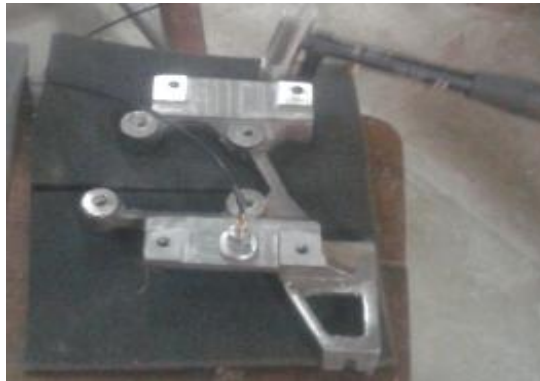
Figure 5.13: Experimental setup for optimized bracket under free-free condition
