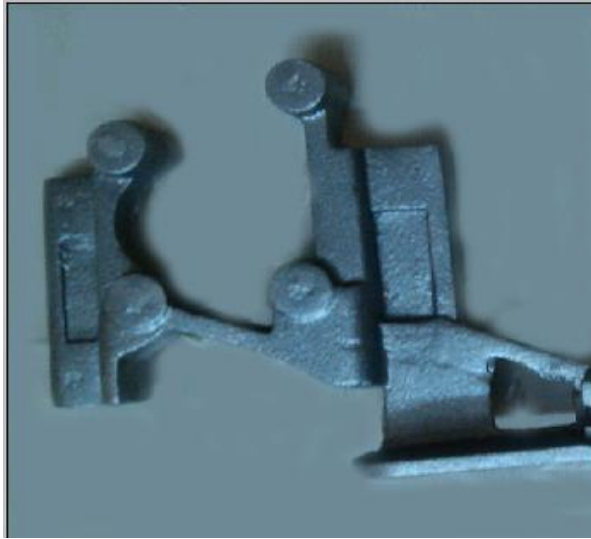
Figure 5.2: Casting of optimized bracket
