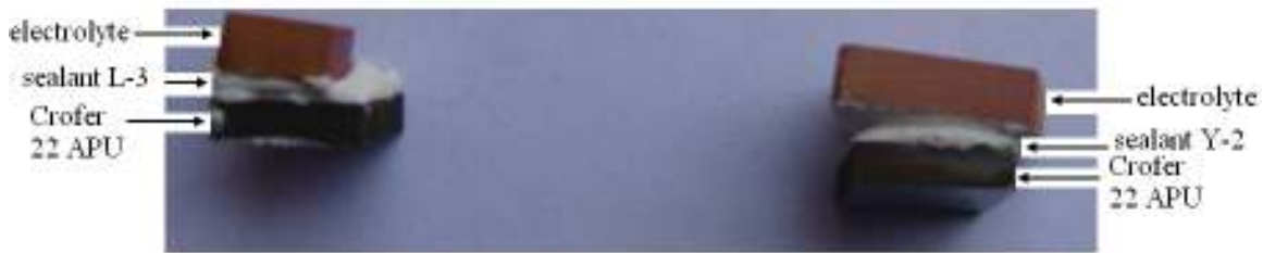
Figure 5.1 Glass sealant sandwiched between Crofer 22 APU and bismuth vanadate
