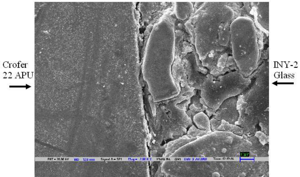
Figure 5.9 (a) SEM micrograph of interconnect (Crofer 22 APU) and sealant (INY-2) heat treated at 800 °C for 100 hrs
