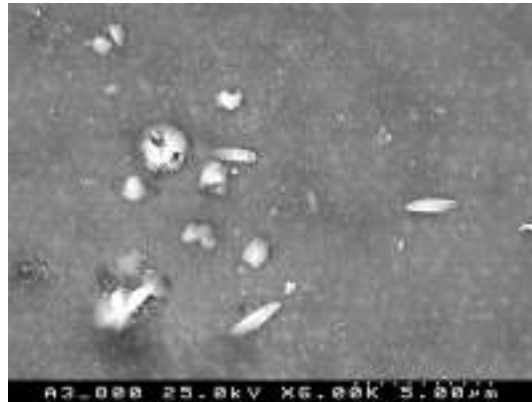
Figure 4.51 SEM micrographs of INA-4 glass sample heat treated at 800 °C for 1 hr
