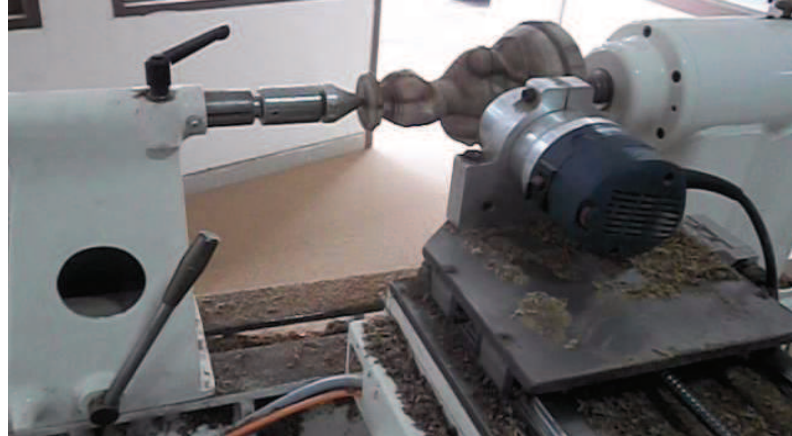
Figure 1.3: Machining of a pseudo-symmetrical part on a CNC router
