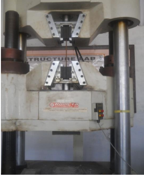
(a) Testing of Steel Bars
