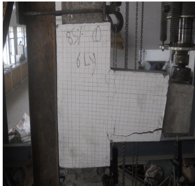
Figure 6.25: Stresses in Ferrocement Retrofitted Beam-Column Joint at Ultimate Load (FE Model vs Experimental)
