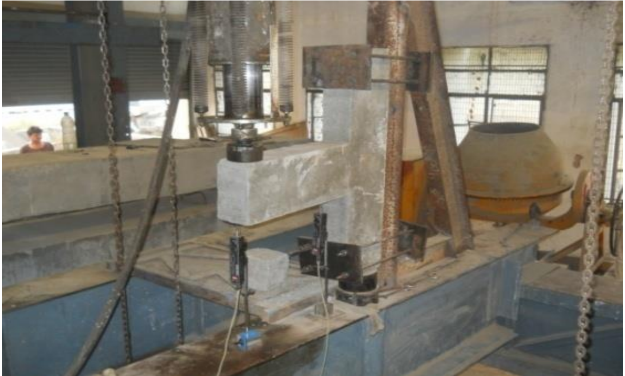
Test Setup for Beam- Column Joints Subjected to Static Load at Beam Tip with LVDT'S At Beam Tip And at 50mm From Column Face
