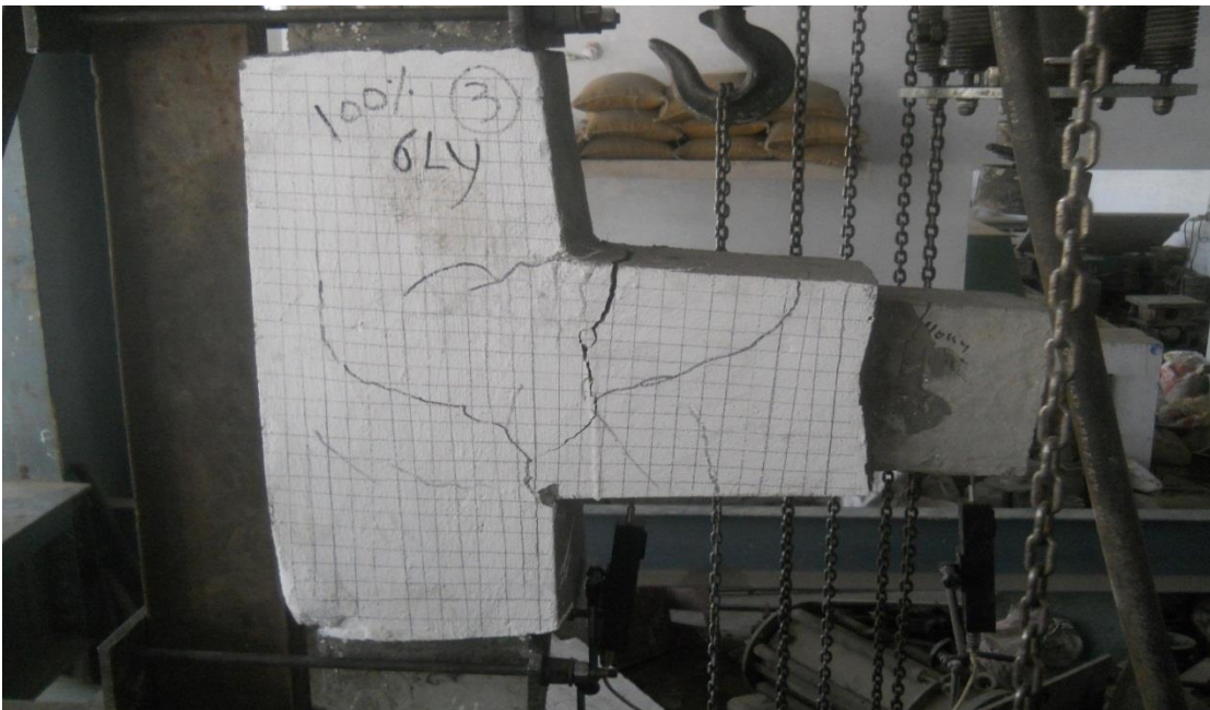
Crack Pattern in Six Layers Retrofitted Joint
