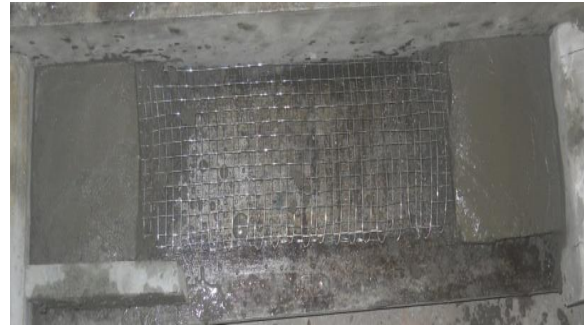
(b) Preparation of Wire Mesh Sample for Testing
