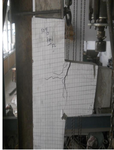
Crack Pattern in Four Layers Retrofitted Joint
