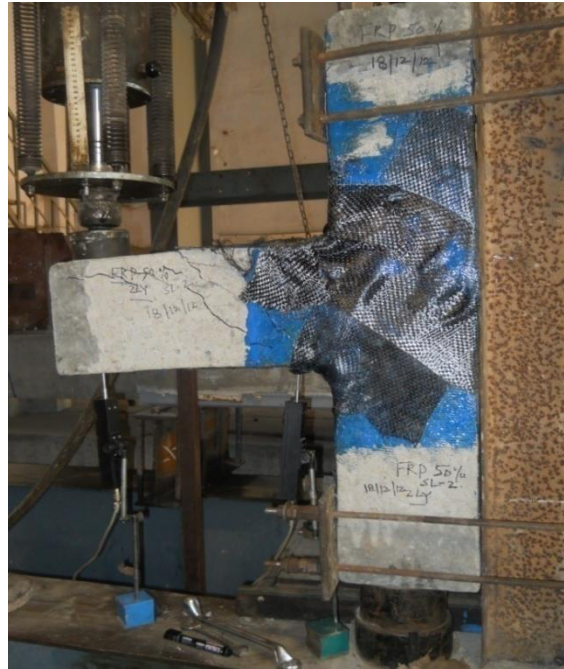
Figure 6.28: Deflected Shape and Cracks of CFRP Retrofitted Beam-Column Joint at Ultimate Load (FEM vs Experimental)
