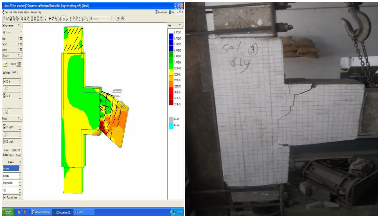
Figure 6.26: Stress Values in Ferrocement Retrofitted Beam-Column Joint at Ultimate Load with Six Layers of Wire Mesh
