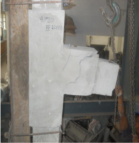
Crack Pattern in Two Layers Retrofitted Joint
