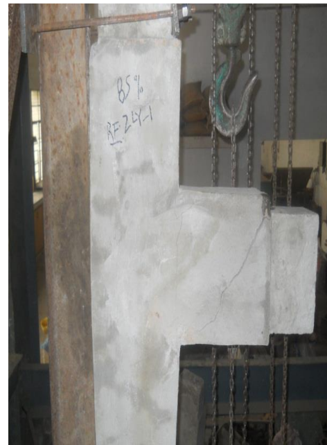
Figure 6.23: Deflected Shape and Cracks of Ferrocement Retrofitted Beam-column Joint at Ultimate Load (FE Model vs Experimental)
