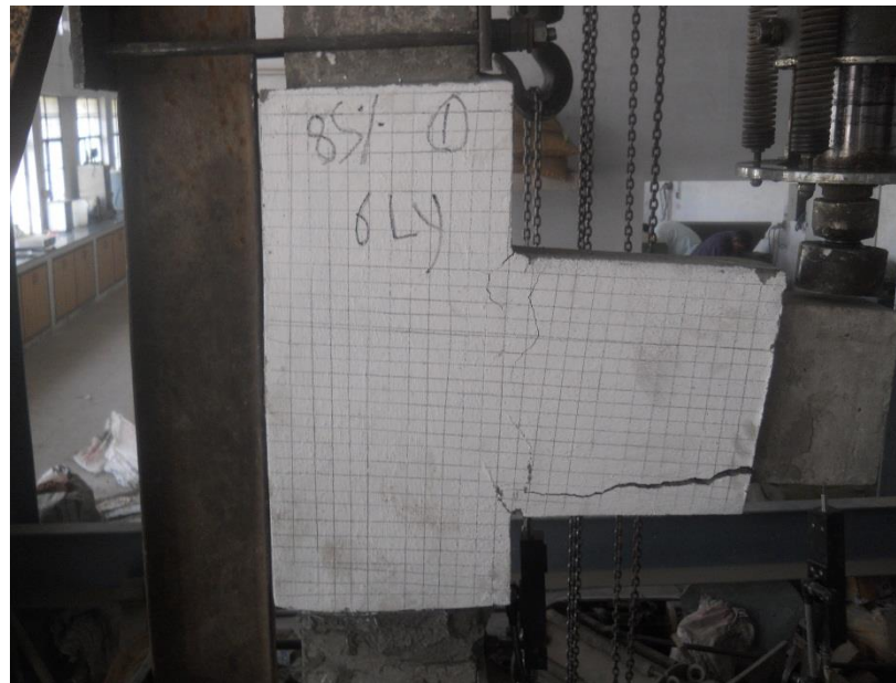
Crack Pattern in Six Layers Retrofitted Joint
