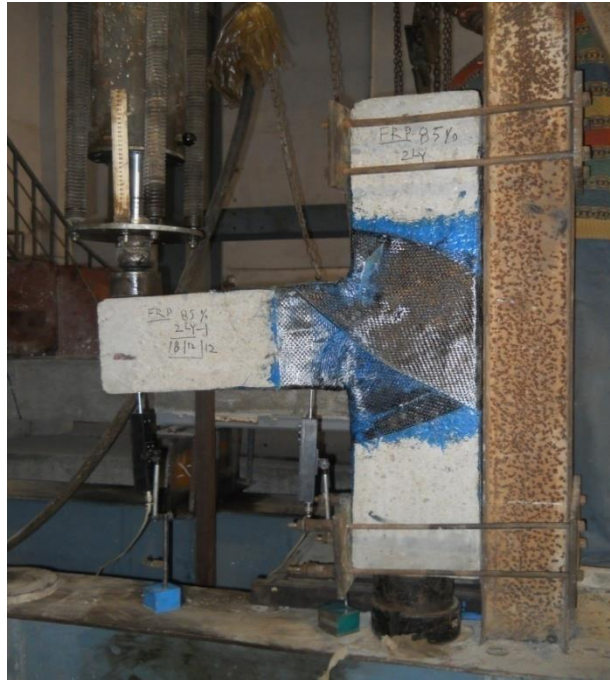
Plate 5.8: Brittle failure of Beam-column Joints Retrofitted with CFRP Jacket Using Two Layers for Stress Level-2
