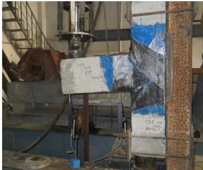
Plate 5.7: Brittle failure of Beam-column Joints Retrofitted with CFRP Jacket Using Two Layers for Stress Level-1
