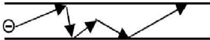
Figure 1.4 Surface scattering phenomena in a copper wire of smaller lateral dimensions [9]
