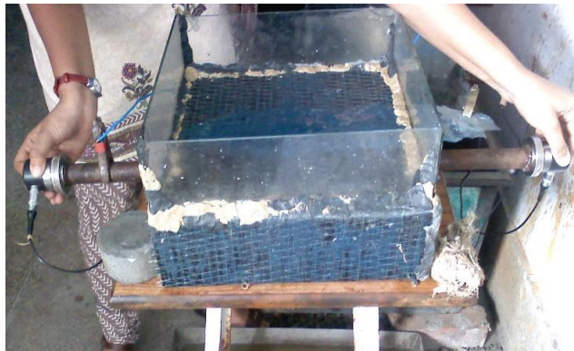
Fig. 6.7 Transducers attached at the Two Ends of Rebar
