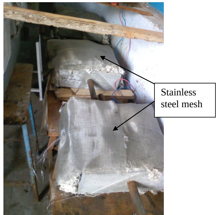
Fig 6.11 Dripping With 5% Nacl Solution
