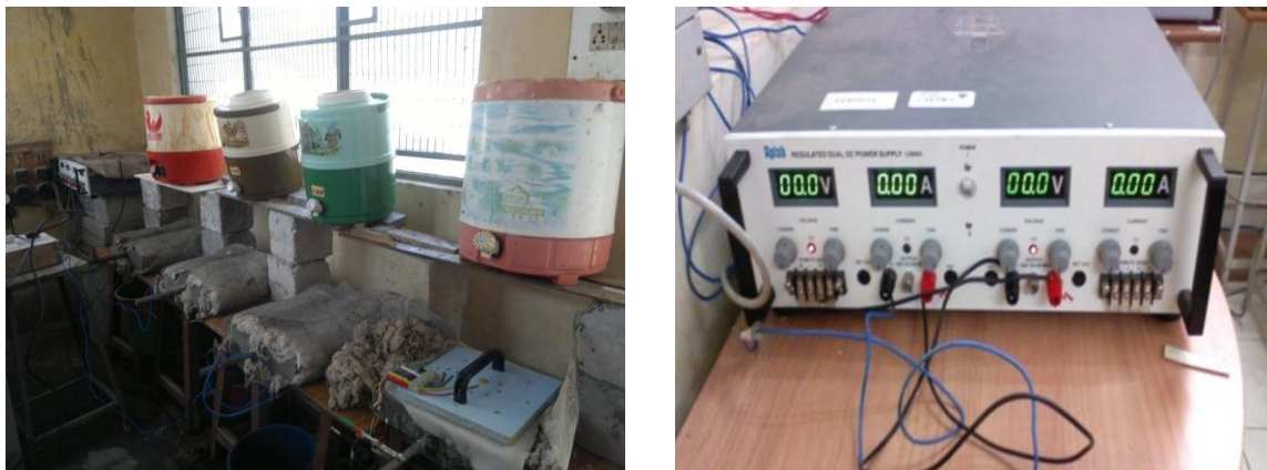
Fig 6.1 Specimens and the Power Supplies Used to Accelerate Corrosion
