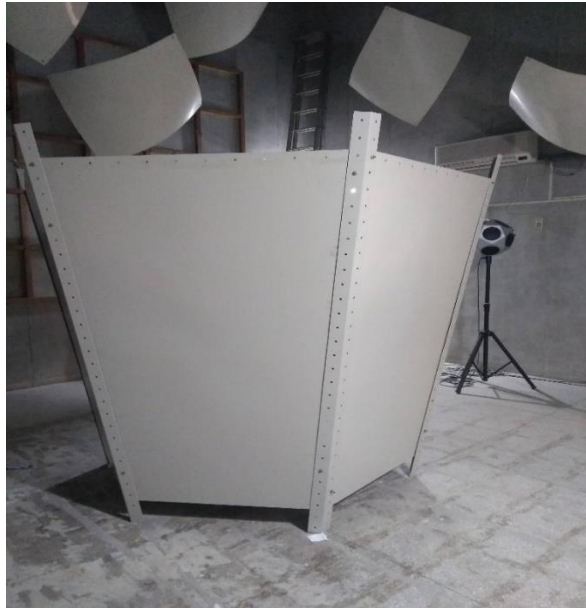
Figure 4.6. SODAR baffle testing in a reverberation chamber
