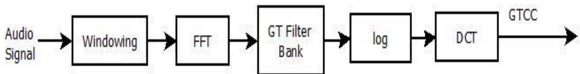
Figure 4.10: Block diagram of GTCC feature extraction technique.
