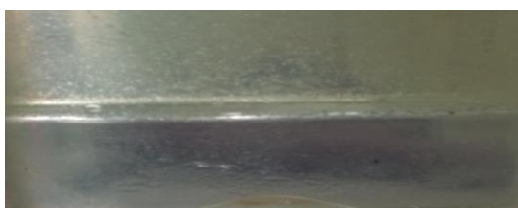
(a) Stratified flow (ST)
