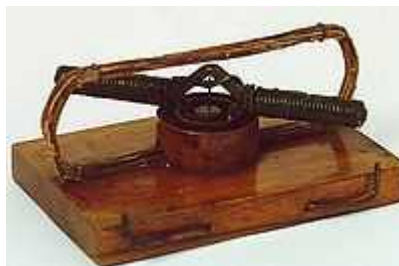
Fig.2.2 Jedlik's "lightning-magnetic self-rotor", 1827
