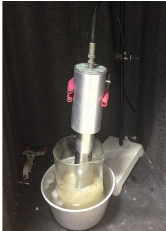
Fig. 4.2 Dispersion of nanoclay into epoxy resin with probe
