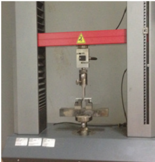
Fig. 4.6 Three point flexural test machine
