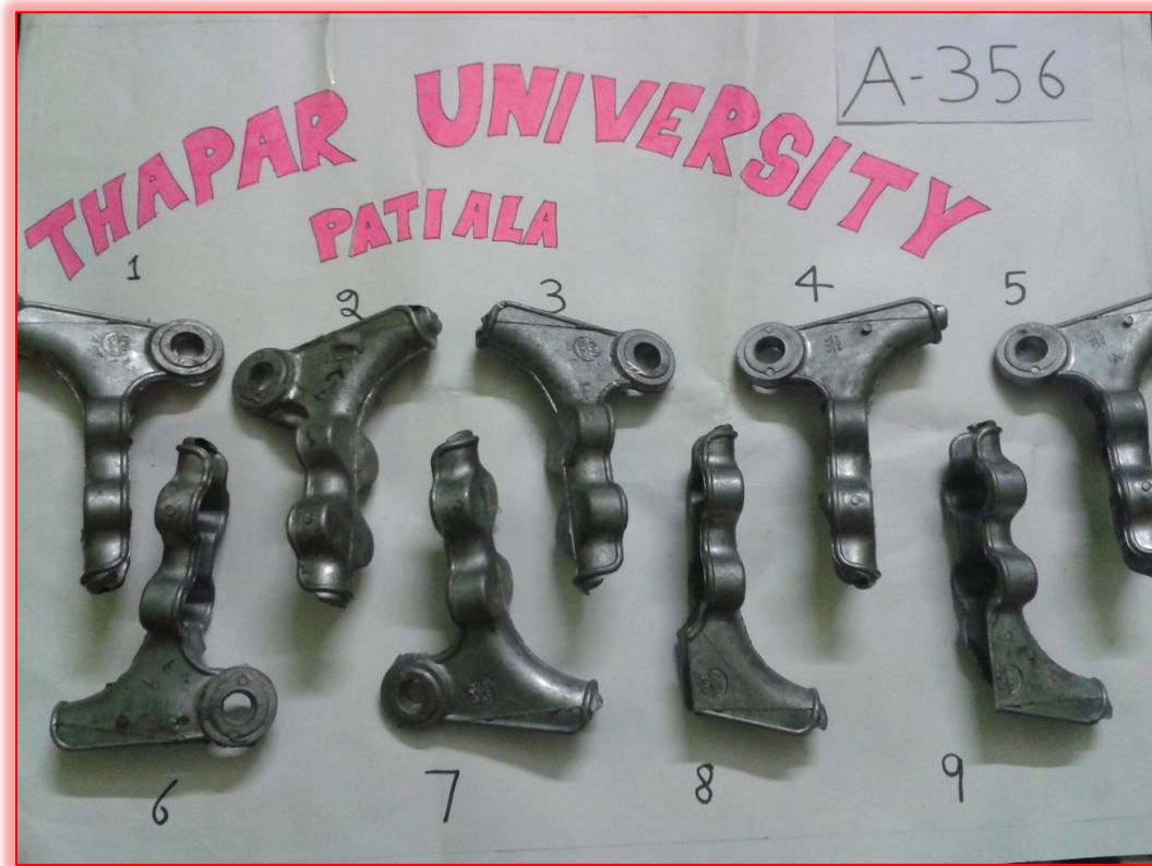
Figure 3.6(a): Final Sample of Material of A-356 after casting
