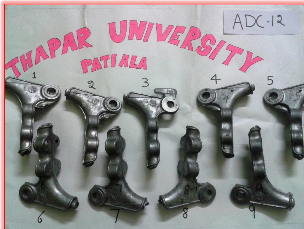
Figure 3.6(b): Final Sample of Material of ADC-12 after casting
