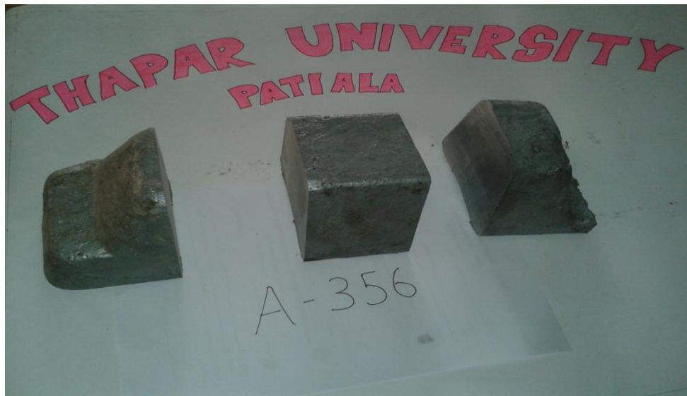
Figure 3.5(a): Raw material of A356 before casting
