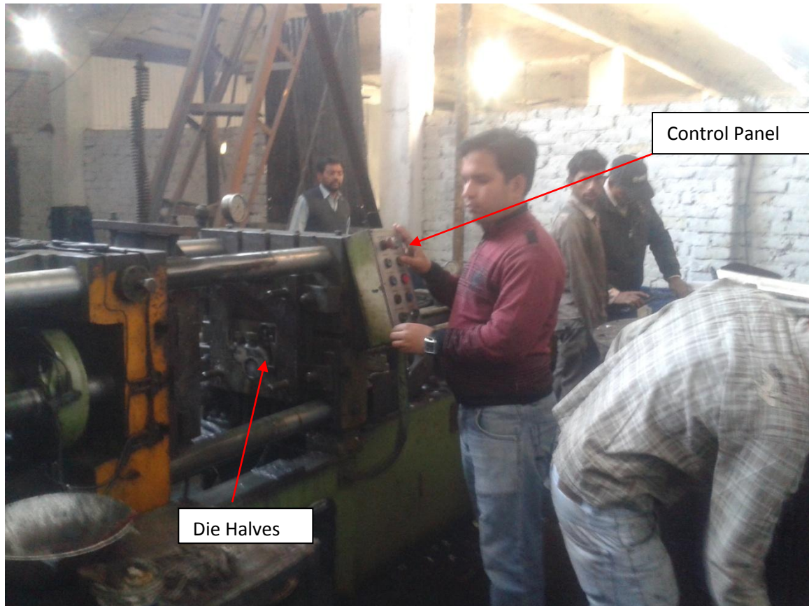
Figure 3.2 High Pressure Cold Chamber Die Casting Machine (120 Tons) at S.L Casting & Allied Industry, D-217, Focal Point, Patiala
