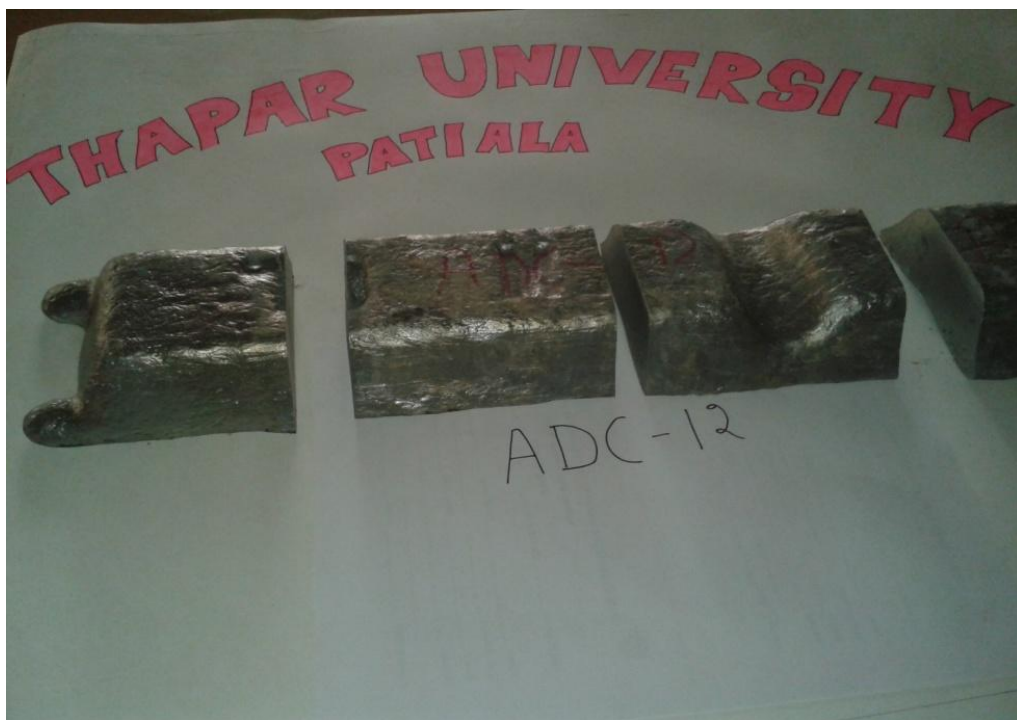
Figure 3.5(b): Raw material of ADC12 before casting
