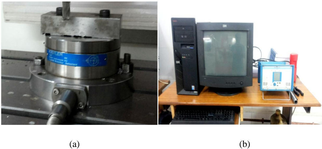
Fig. 5.5 (a) Kistler piezoelectric dynamometer (b) desktop and application software
