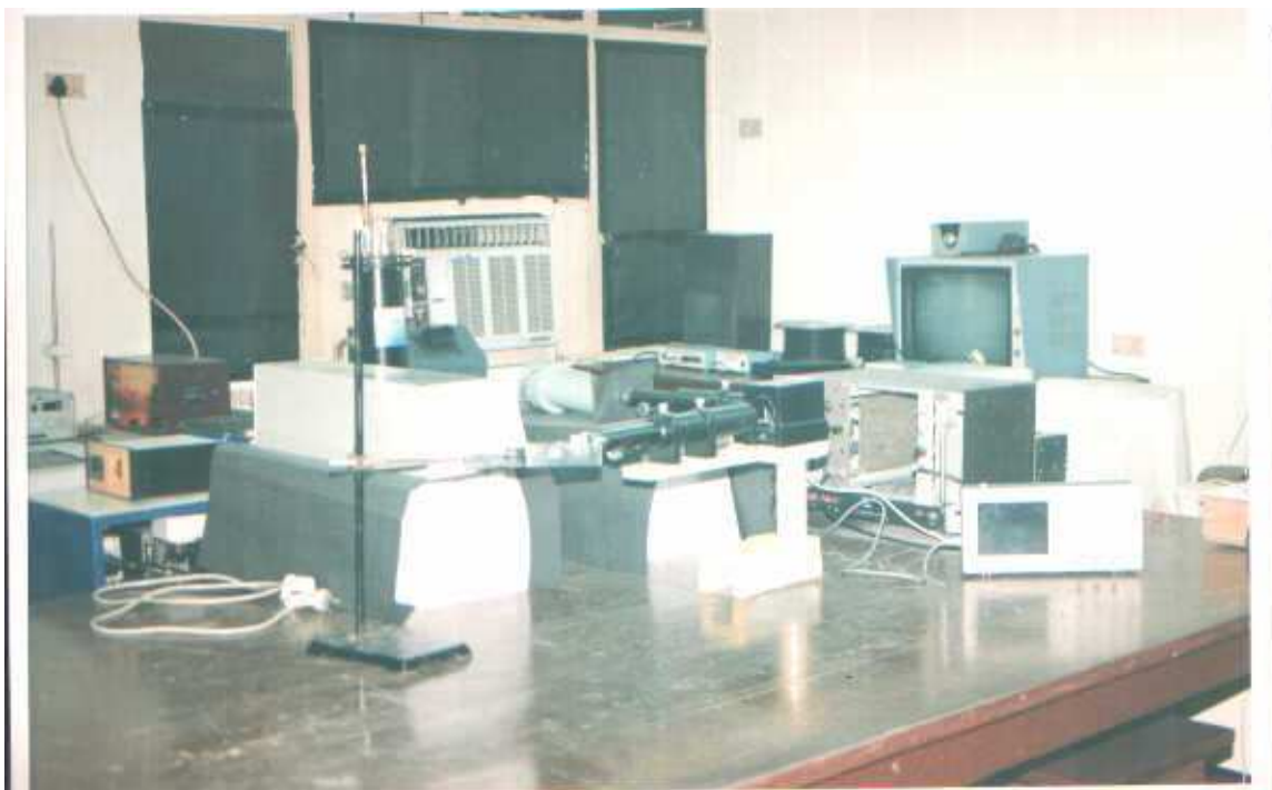
Fig.5-Photograph of experimental set-up for life-time measurement studies at room temperature.
