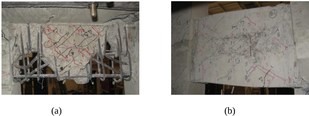
Figure 2.5. Reinforced concrete (a) and HPFRC (b) coupling of beams at completion of testing (Lequesne et al., 2013)
