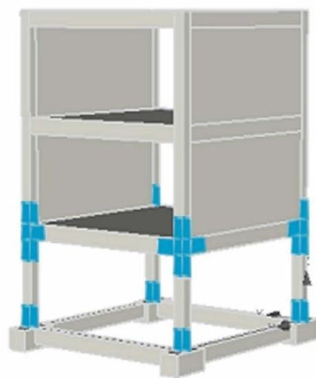
Figure 6.15 View of FE model of Retrofitted Frame
