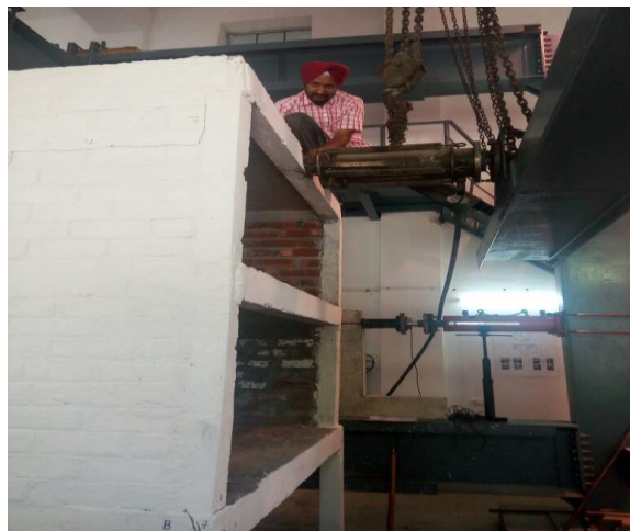
Figure 3.38 loading jack at top floor
