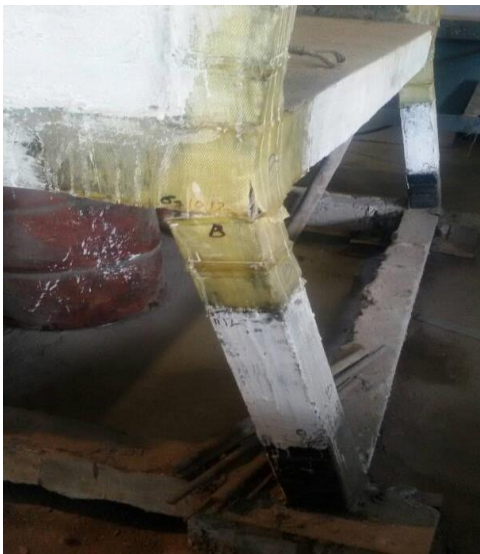
Figure 6.23 Deflected FRP retrofitted experimental and FE frame.
