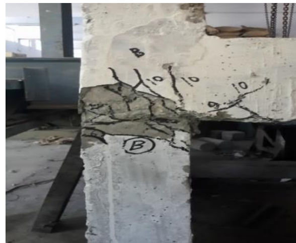
(b) Column-beam joint in B
