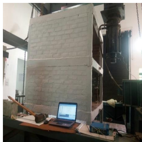
Figure 3.37 ECC Restrengthened Frame
