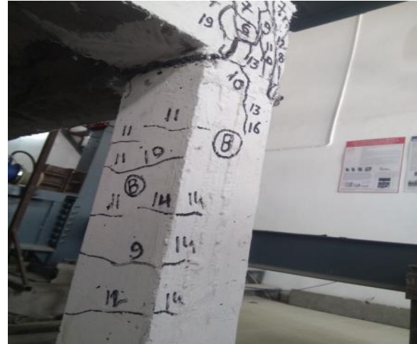
(b) Beam-Column Joint B
