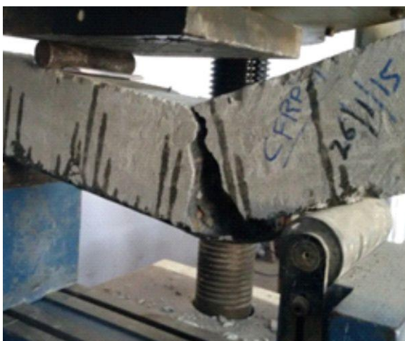
Figure 3.17 CFRP Retrofitted Prisms
