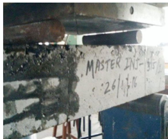
Figure 3.18. Reconnected prism using epoxy
