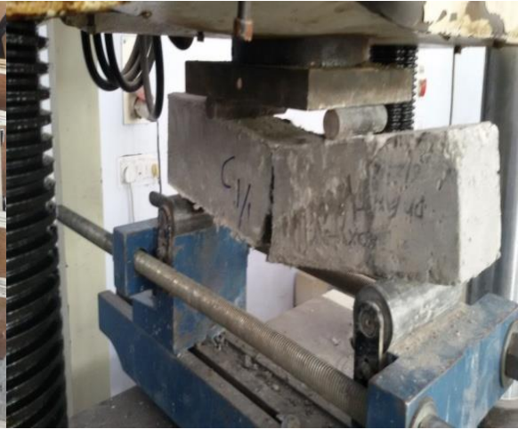
Figure 3.29 Testing of reconnected prisms
