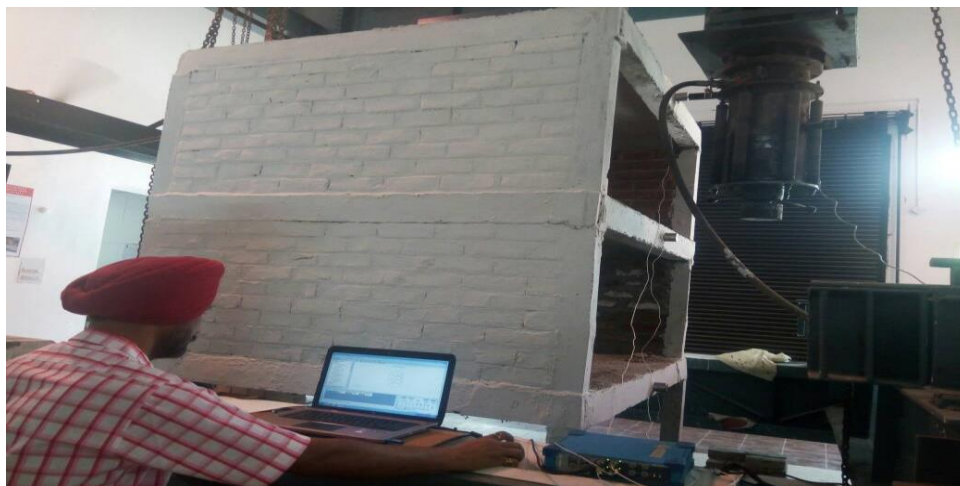
Figure 3.45 Vibration testing of frame at laboratory
