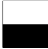
Figure 4.1 (b) Haar wavelet for gradient calculation in y-direction [12]
