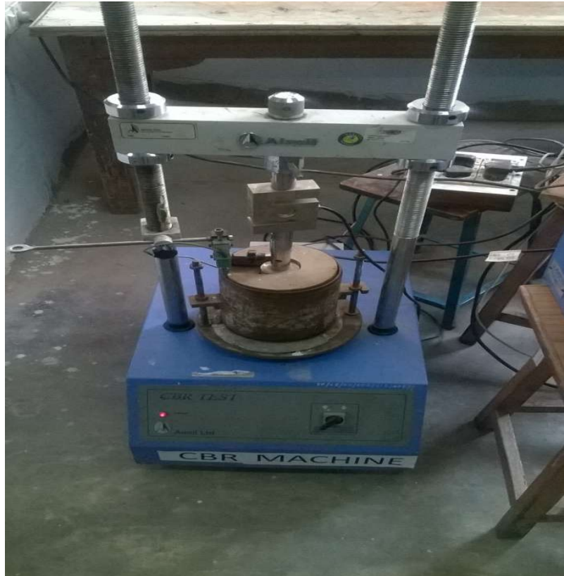
Plate 3.4: Compacted Sample at RBI Grade81: Soil in a Mould
