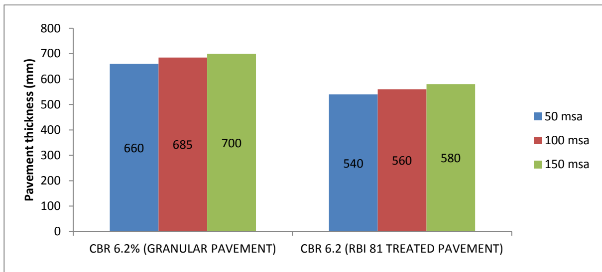
Graph 5.3: Comparison between granular CBR 6.2% at 0% RBI Grade 81 dosage and cemented CBR 6.2% at 0% RBI Grade 81 dosage w.r.t pavement thickness
