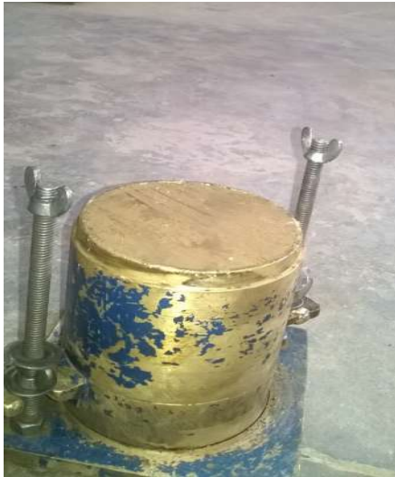
Plate 3.2: compacted sample in mould
