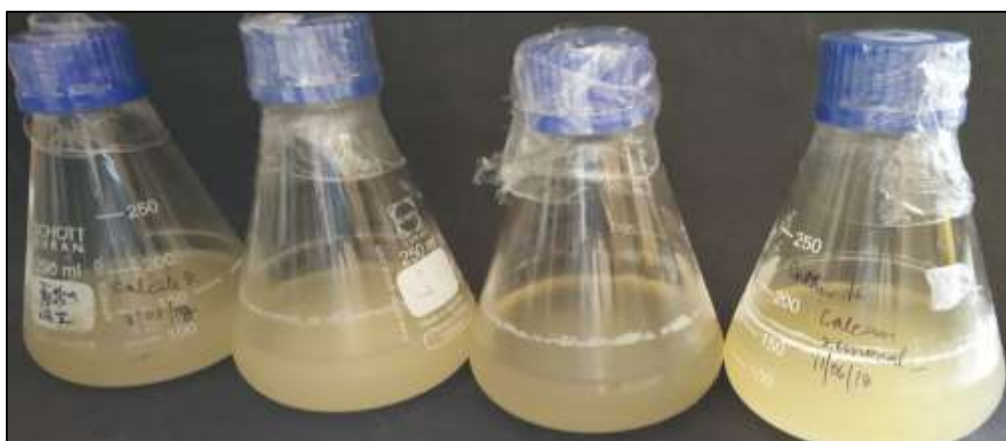
Figure 4.7: Calcium carbonate precipitated on the walls of culture flask.
