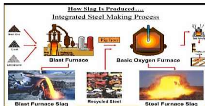
Figure 2.1: The basic process of generation of slag and its kinds (source: Tiwari et al, 2016).
