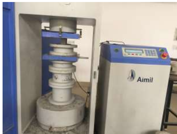
Figure 3.3: Autocompression testing machine COMPTEST 3000.
