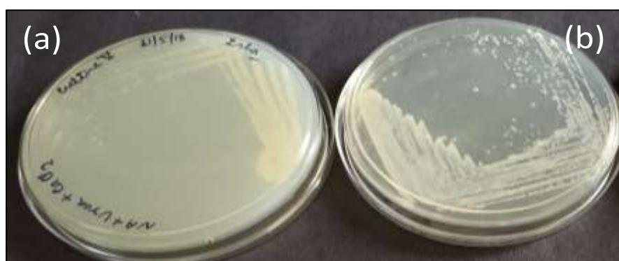
Figure 4.9: Calcium carbonate precipitation (a) yellow colonies of bacterial strain on NA+ urea+ \text{CaCl}_2 plates, (b) white colonies of bacterial strain on NA plate (control)
