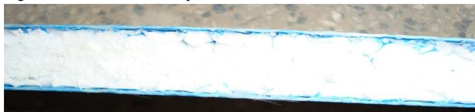
Fig.5.9 Shows condition of specimen of 16mm core thickness 30% UFL at natural degradation
