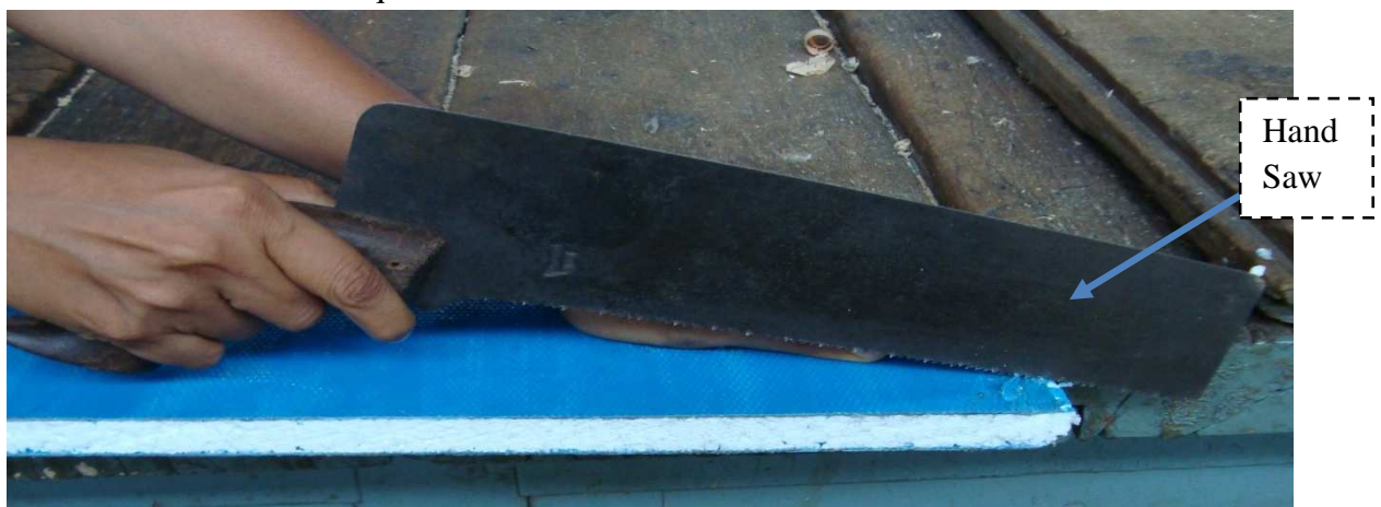
Fig.4.15 Cutting of specimen with the help of Hand Saw
