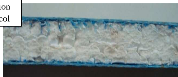
Fig.5.7 Shows condition of specimen of 16mm core thickness at 30% UFL
