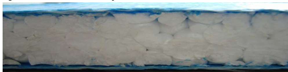
Fig.5.14 Shows condition of specimen of 16mm core thickness 30% UFL at natural degradation
