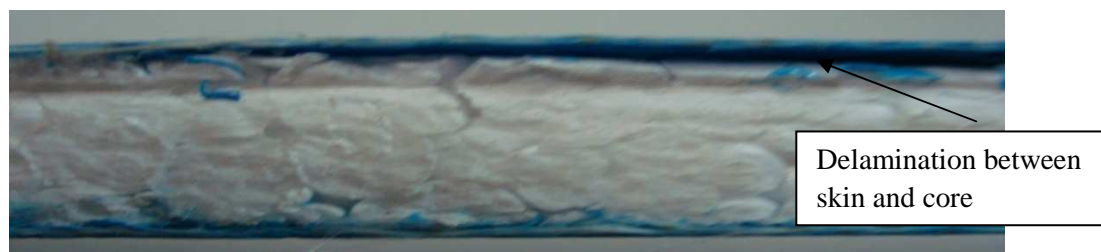
Fig.5.13 Shows condition of specimen of 16mm core thickness at 70% UFL
