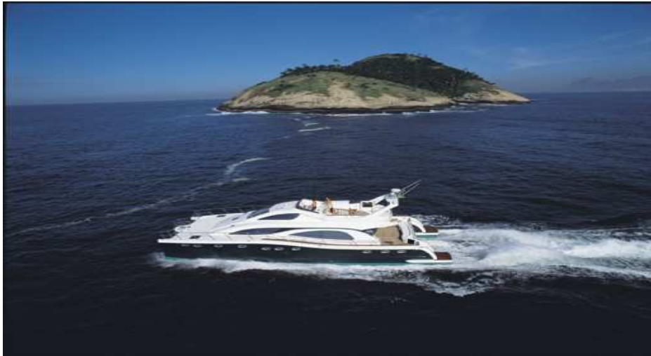
Fig.1.14(b) The Cat190 is a motor powered oceanic luxury catamaran, with hulls and glass fibre structure with Sandwich of foam or polystyrene. [21]
