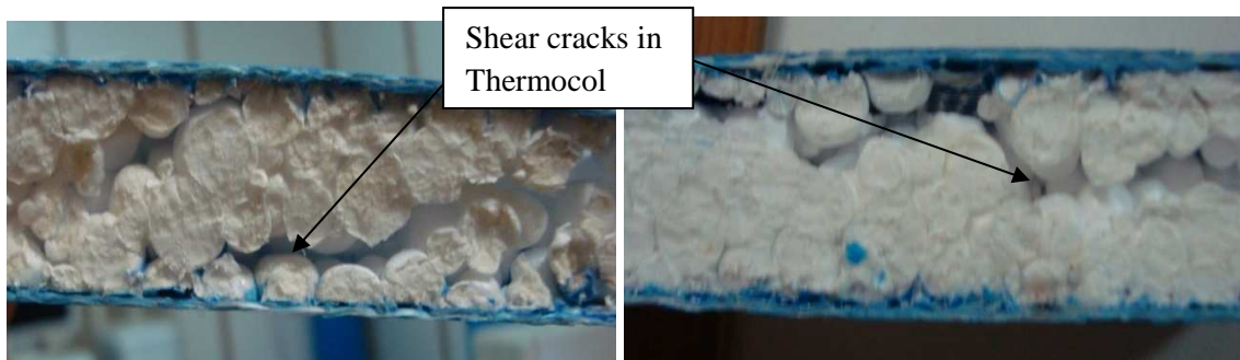
Fig.5.11 Shows condition of specimen of 16mm core thickness at 30% UFL
