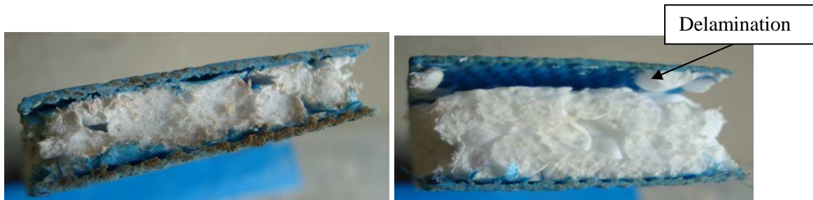
Fig.5.23 Shows condition of specimen of 8mm core thickness at 70% UFL
