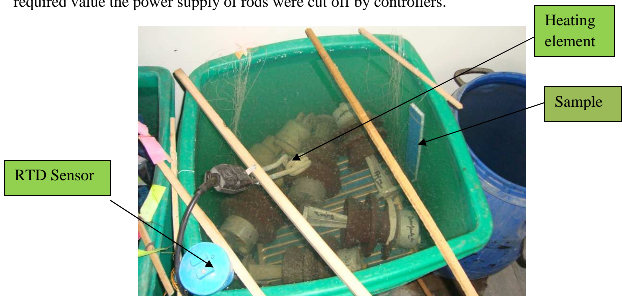
Fig. 4.4 Heating Element and RTD sensor in a tank
