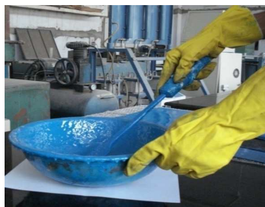
Fig.4.14 Hand mixing of both base and hardener
