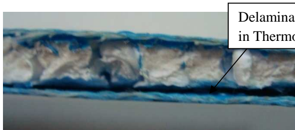
Fig.5.6 Shows condition of specimen of 8mm core thickness at 70% UFL
