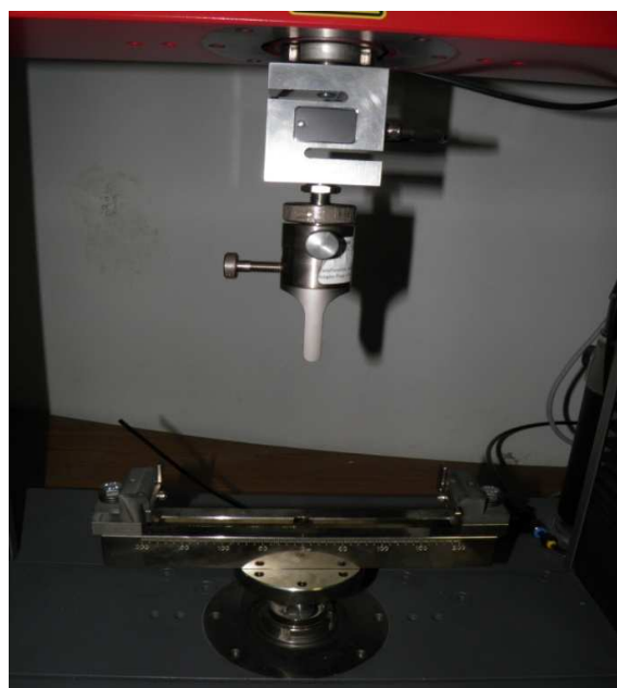
Fig. 4.21 Flexural Testing setup
