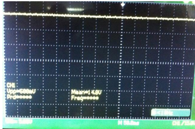
Figure 5.8: Full wave rectifier output waveform
