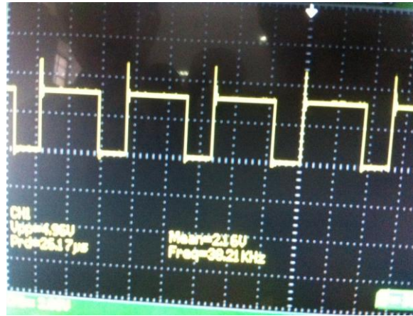
Figure 5.4: NE 555 Timer IC output waveform of transmitter circuit
