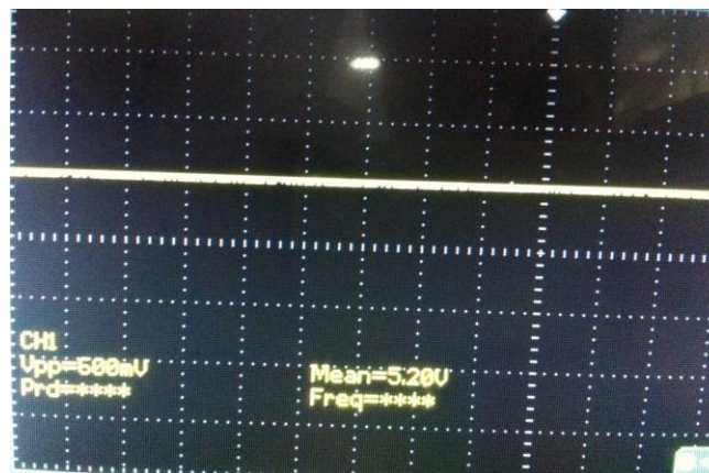
Figure 5.9: output waveform of IC 7805
