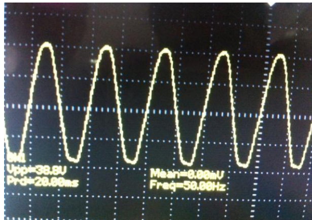
Figure 5.7: Transformer output waveform
