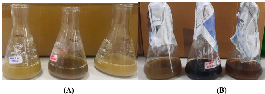
Fig.5. Before (A) and after (B) steam explosion pre-treatment
