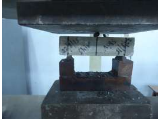
Fig. 3.7: Flexural Strength Testing of Specimen under UTM by Centre Point Loading
