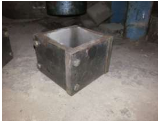
Fig. 3.2: Cube Specimens of Size 70.6 mm x 70.6 mm x 70.6 mm
