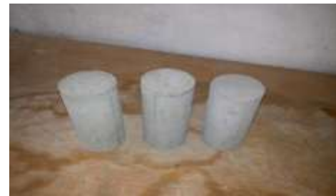
Fig. 3.9 (b): Casted Cylindrical Specimens of Size 100 mm x 200 mm
