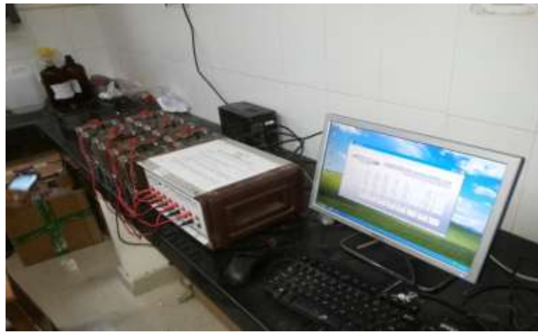
Fig.3.13: Rapid Chloride Permeability Test Setup
