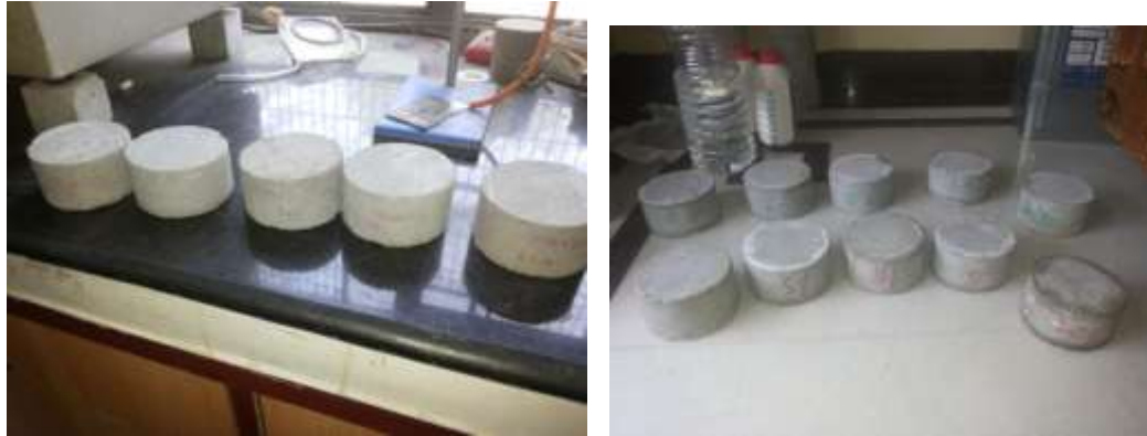
Fig. 3.11: Cylindrical Specimens of Size 51 mm x 100 mm
