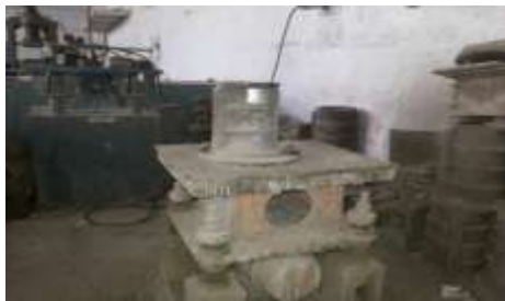
Fig. 3.9 (a): Cylindrical Mould for Specimens of Size 100 mm x 200 mm
