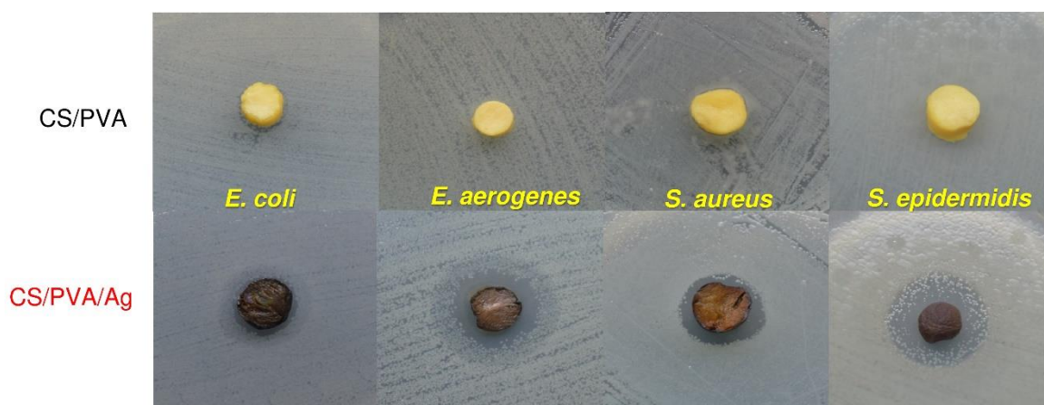
Figure 4.6 Disc diffusion tests for comparing the antibacterial activity of hydrogel before and after immobilizing silver nanoparticles (CS/PVA/Ag) in solid media.
