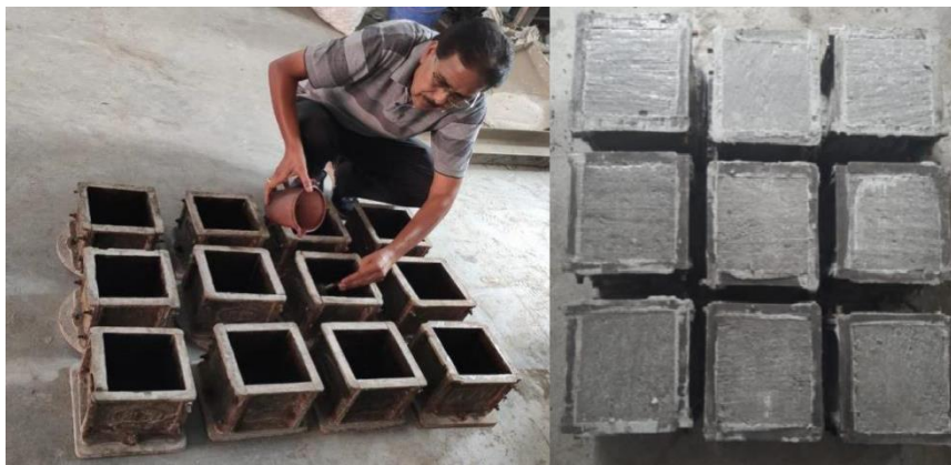
Fig 3.7: (a) Greasing and oiling of moulds (b) Casting of concrete mix
