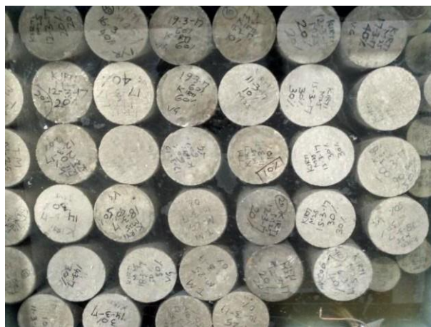
Fig. 3.8: Curing of concrete specimens in the temperature-controlled curing tank
