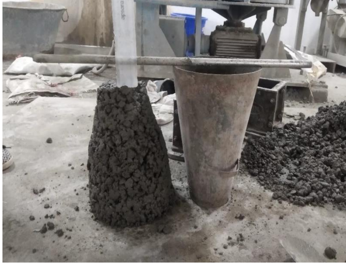
Fig. 3.9: Slump test apparatus
