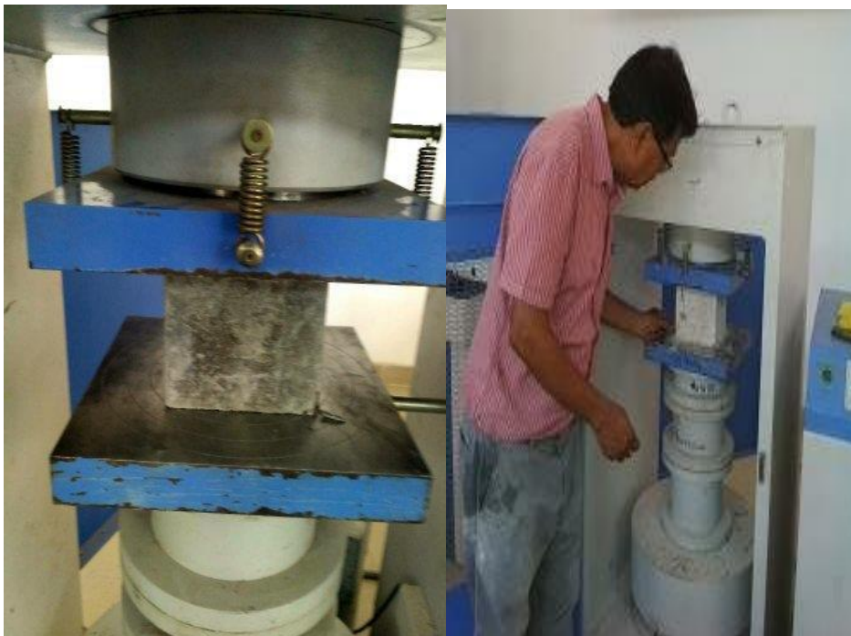
Fig. 3.10: (a) compression testing machine, (b) Compression test in progress
