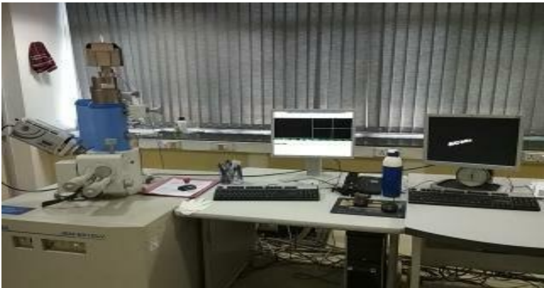
Fig. 3.17: Experimental set up for SEM and EDS spectroscopy
