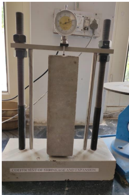
Fig. 4.28: Unrestrained drying shrinkage test set-up
