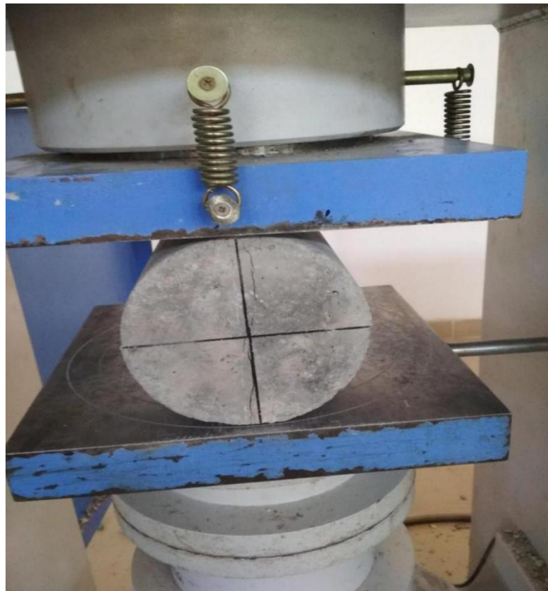
Fig. 3.11: Test set up and crack development in split tensile strength
