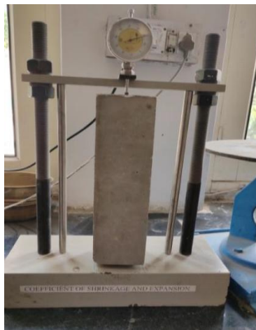
Fig. 3.16: Unrestrained drying shrinkage test set-up
