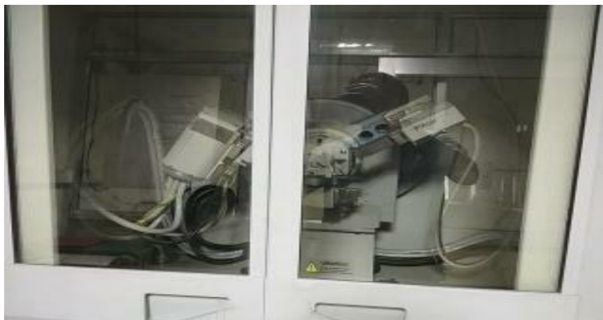
Fig. 3.18: Experimental set up for X-Ray diffraction (XRD) instrument
