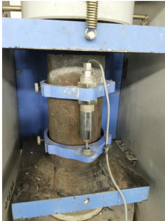
Fig. 3.9: Experimental set up for measuring modulus of elasticity of concrete
