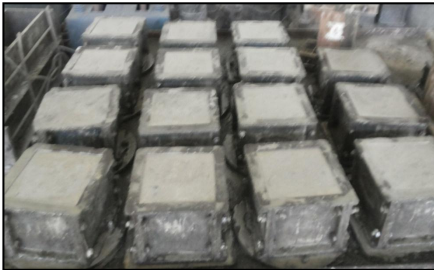
Fig.3.2: Casting of concrete cubes for compressive strength
