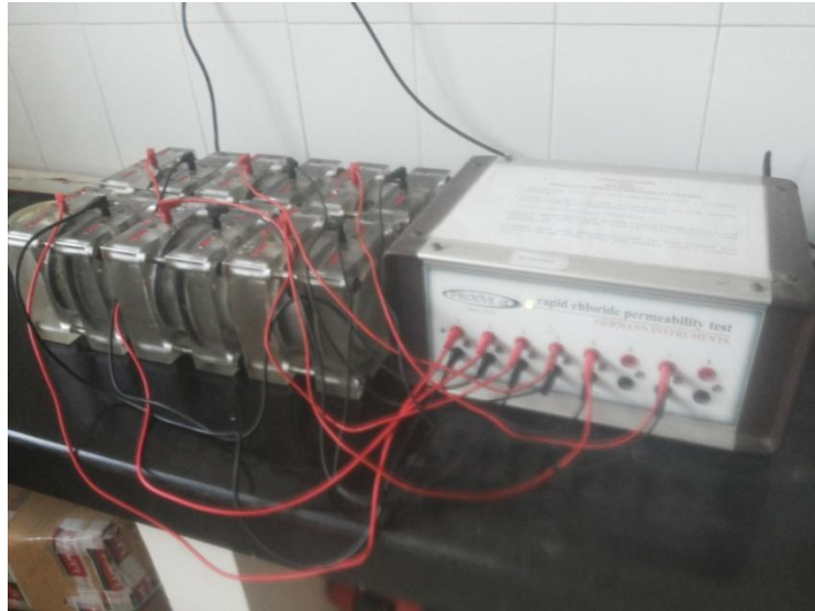
Fig. 3.17: Experimental set up for measuring chloride ion penetration
