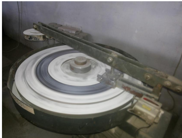
Fig. 3.16: Experimental set up for measuring abrasion resistance of concrete
