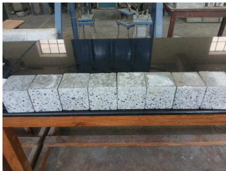
Fig. 3.14: Deterioration of specimens after 7 days of immersion in 3% sulphuric acid solution (Concrete 'B')
