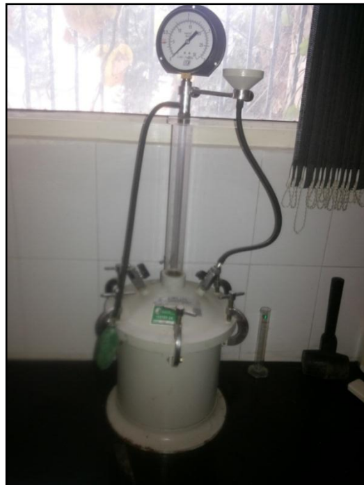
Fig 3.4: Experimental set up for measuring air content in fresh concrete
