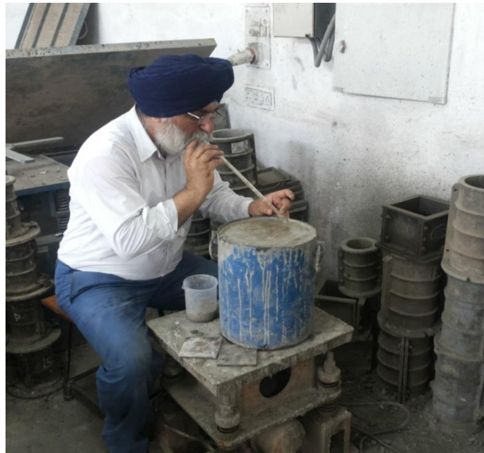
Fig. 3.5: Experimental set up for collection of bleeding water from the surface of concrete
