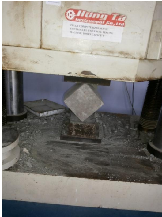
Fig. 3.8: Experimental set up for measuring Splitting tensile strength of concrete
