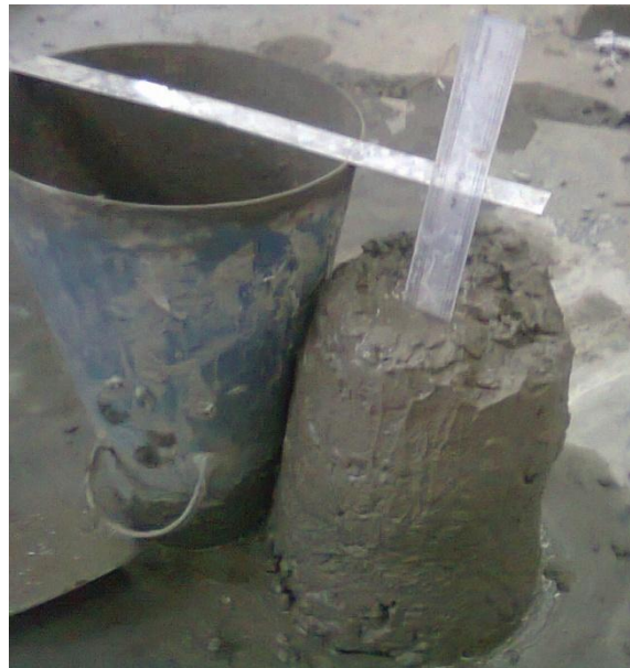
Fig. 3.3: Experimental set up for measuring slump of fresh concrete
