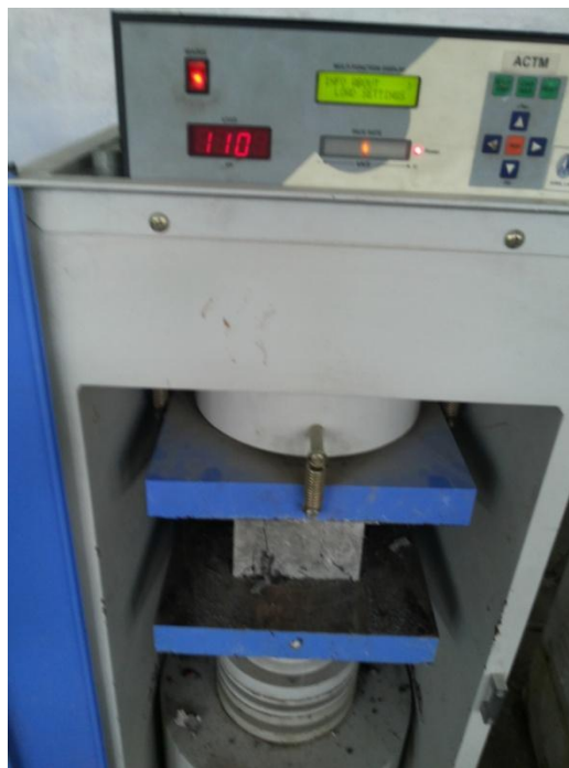
Fig. 3.7: Compression testing machine (Capacity 3000 kN)
