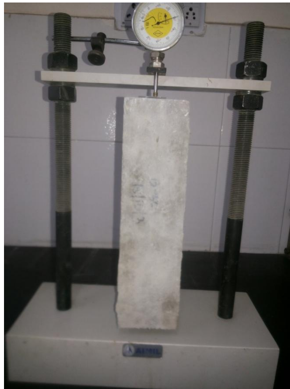
Fig. 3.11: Experimental set up for measuring length change
