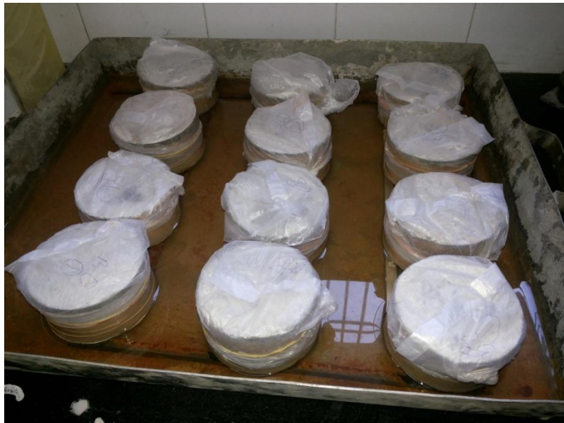
Fig. 3.6: Experimental set up for measuring sorptivity of concrete
