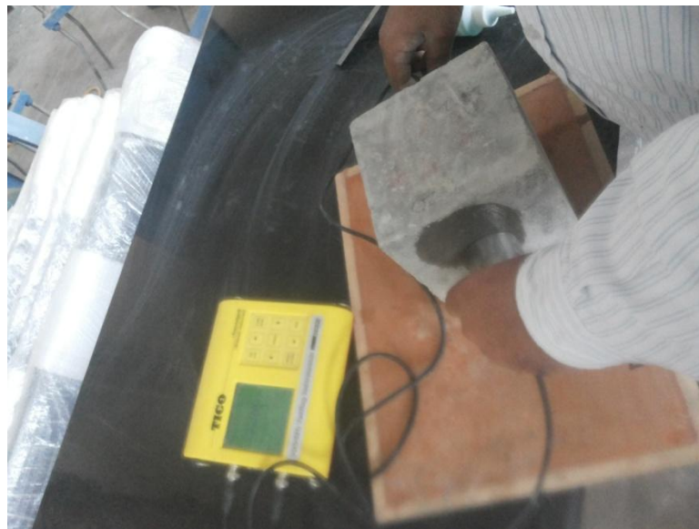
Fig. 3.10: Experimental set up for measuring pulse velocity through concrete
