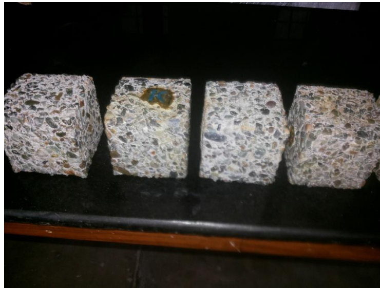
Fig. 3.15: Deterioration of specimens after 84 days of immersion in 3% sulphuric acid solution
