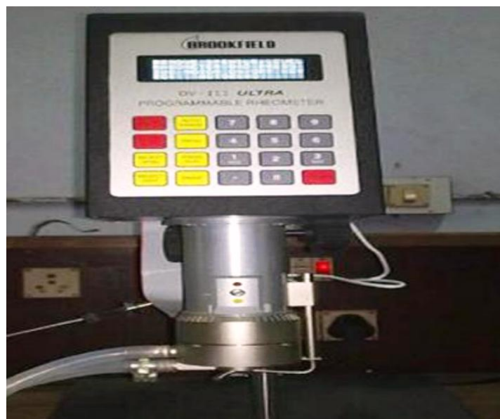
Figure 4.12: Pictorial view of brookfield viscometer
