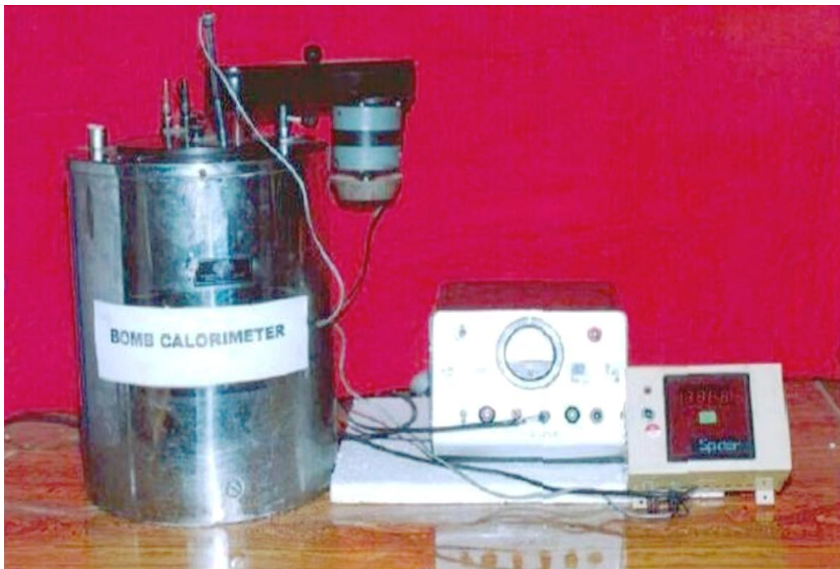
Figure 4.10: Pictorial view of bomb calorimeter
