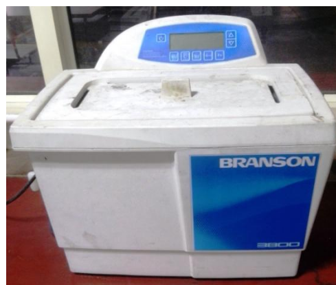
Figure 4.9: Pictorial view of ultrasonic bath
