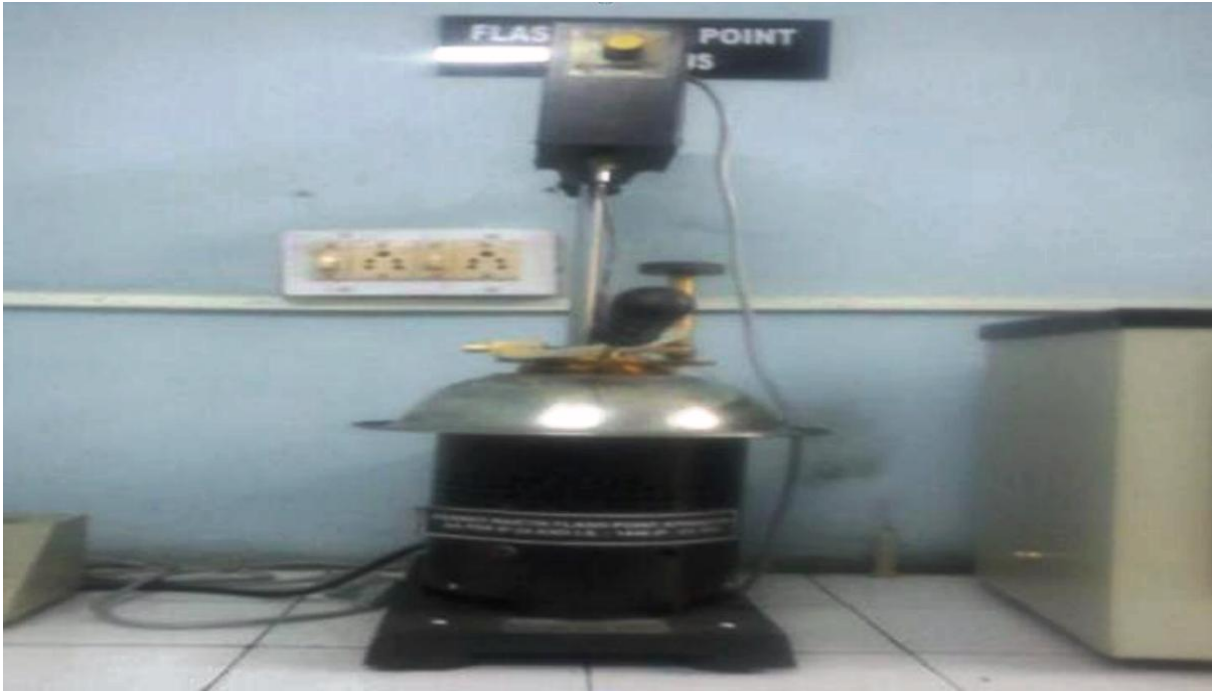
Figure 4.11: Pictorial view of pensky martin (closed cup) apparatus
