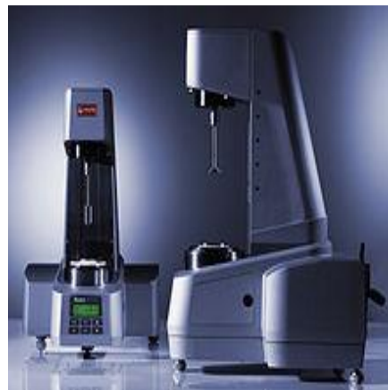
Fig. 1.15: Rotational rheometer having plate/cone measuring system (right) and cylindrical measuring system (left)
