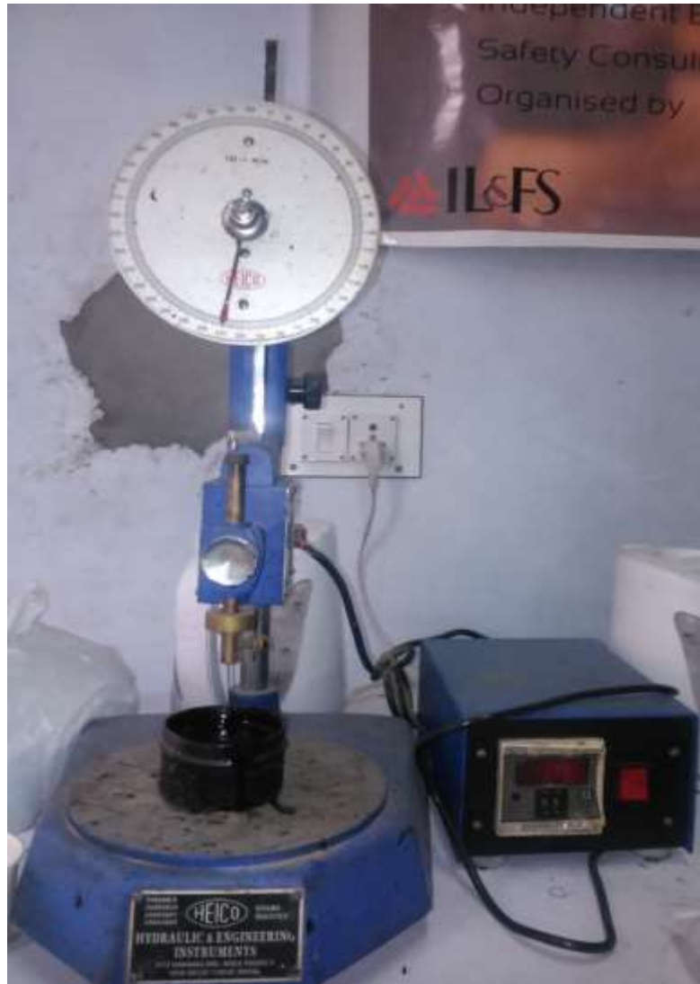
Plate 3.7: Penetration test apparatus
