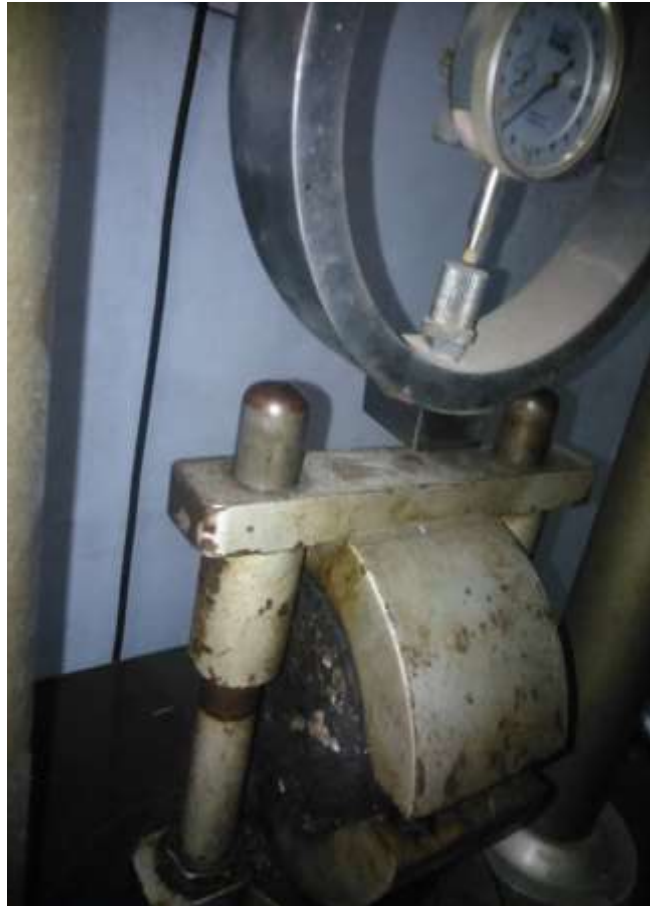
Plate 3.5: Specimen testing in Marshall Stability machine
