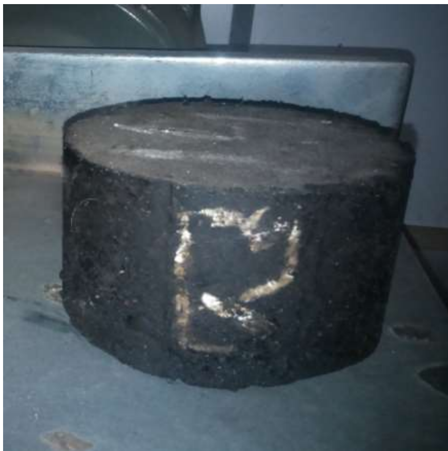
Plate 3.4: Samples extracted from Marshall mould
