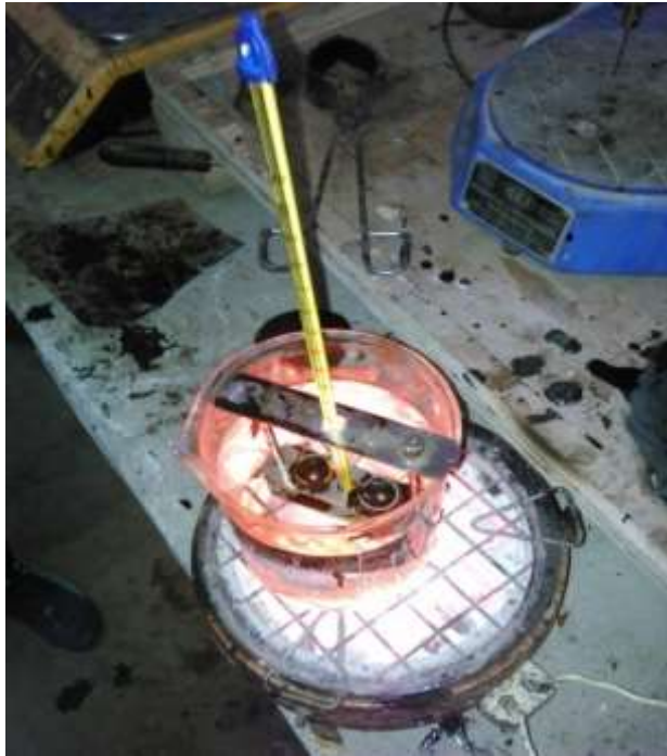
Plate 3.8: Softening point test apparatus
