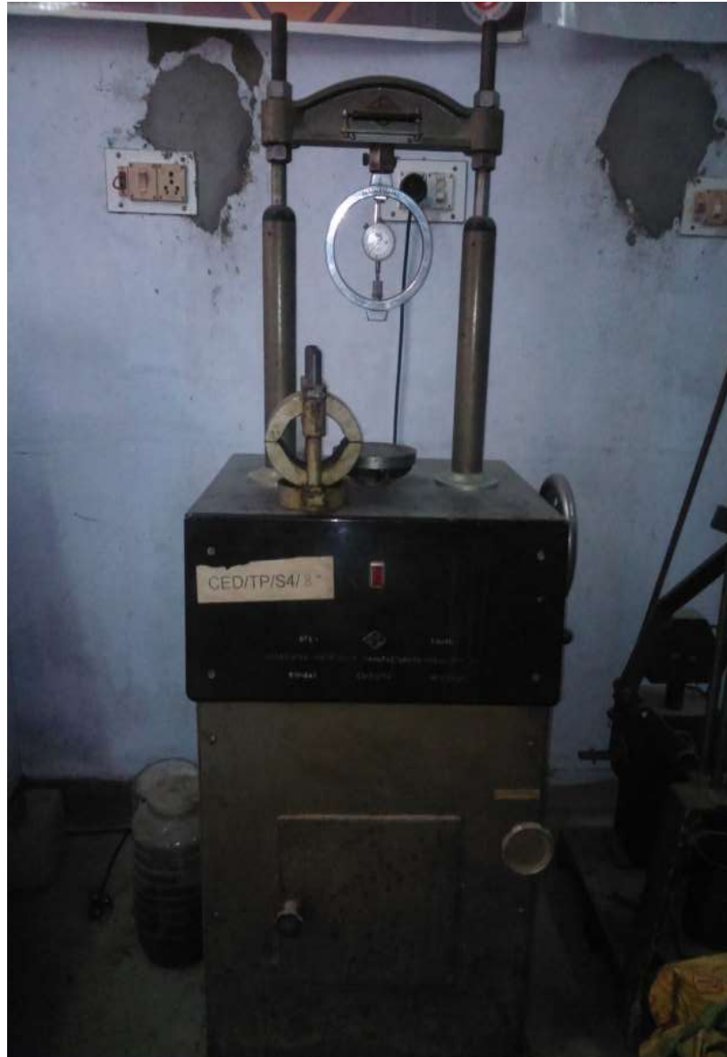
Plate 3.3: Marshall stability testing machine
