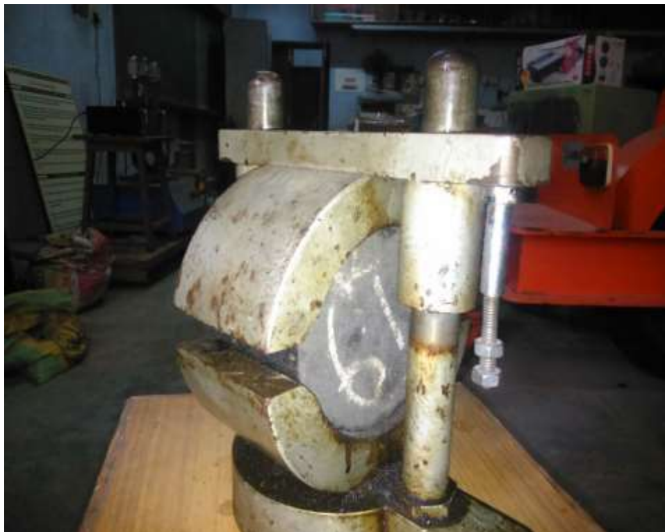
Plate 3.6: Testing head of Marshall stability machine
