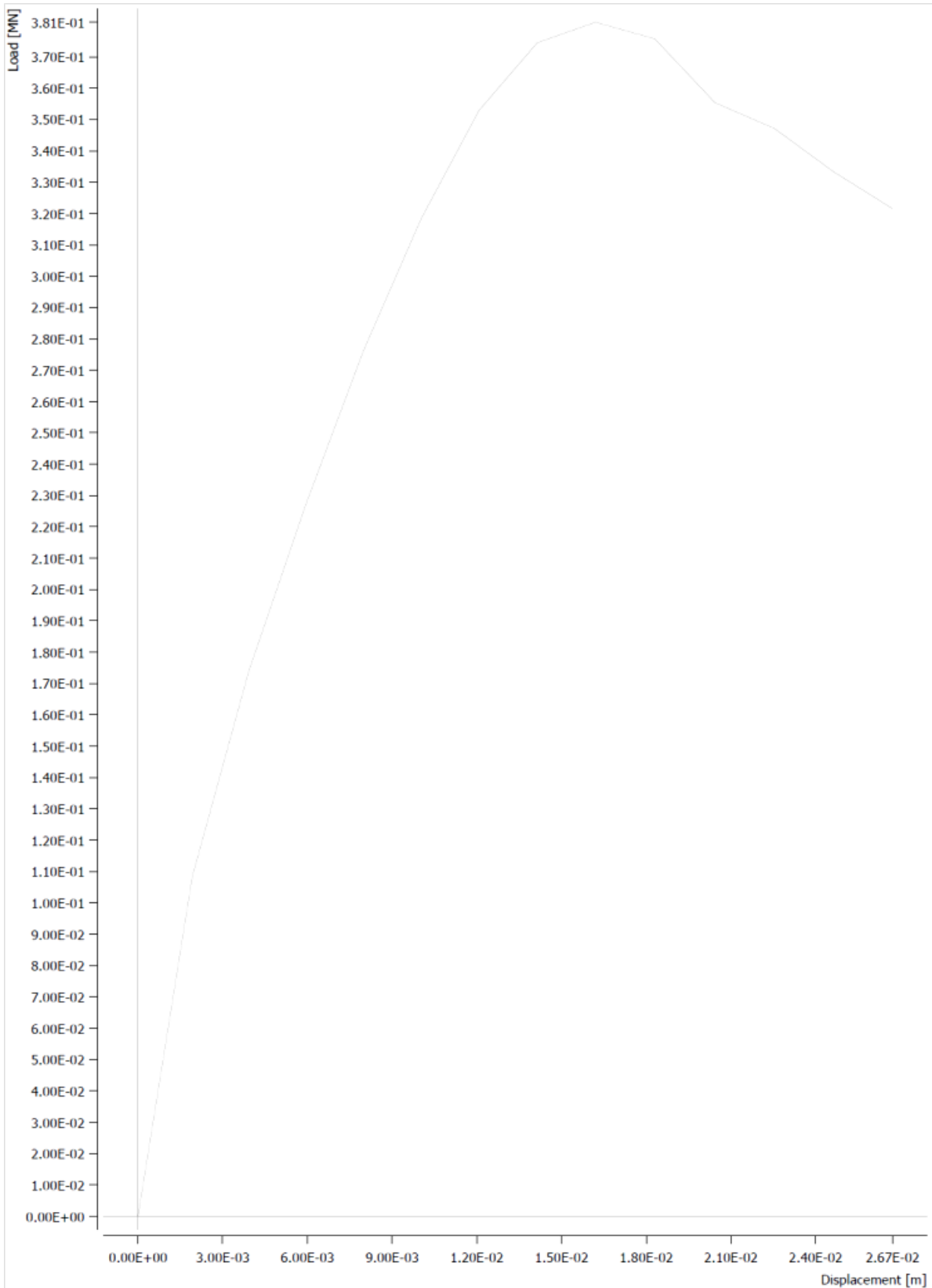
Figure-5.12, Load displacement curve for RC Single Strut frame (Pauley & Prisley) under Monotonic Loading.
