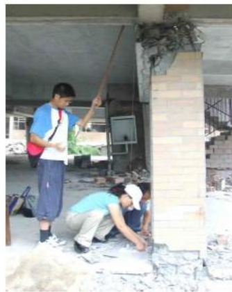
Fig-2.2(b) Measuring column drift
