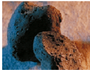
Fig2.5: Showing porous dense shell of filtralite media.
