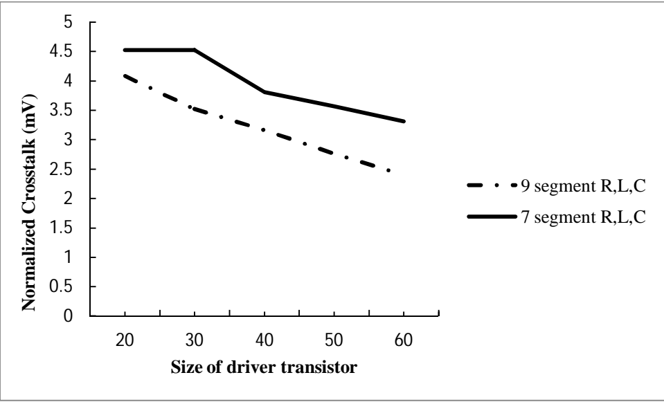
Figure 5.9 Normalized crosstalk noise for 9 segment RLC and 7 segment RLC versus different size of driver transistor in CNT.
