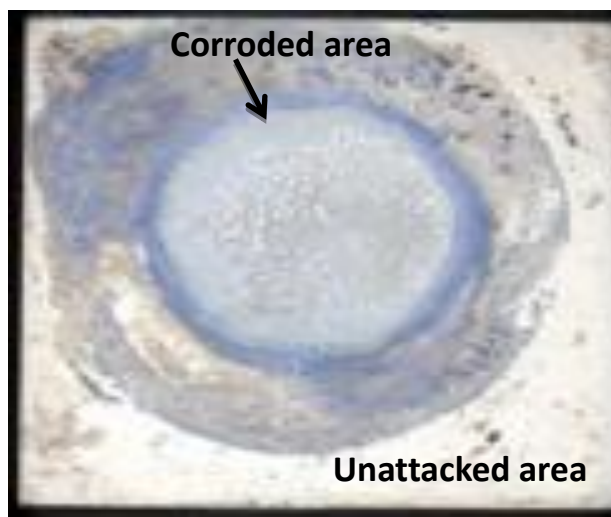
Fig. 4.162: Photographs of surfaces of HSLA steel samples before and after corrosion testing for 24 h in 3.5% NaCl solution.
