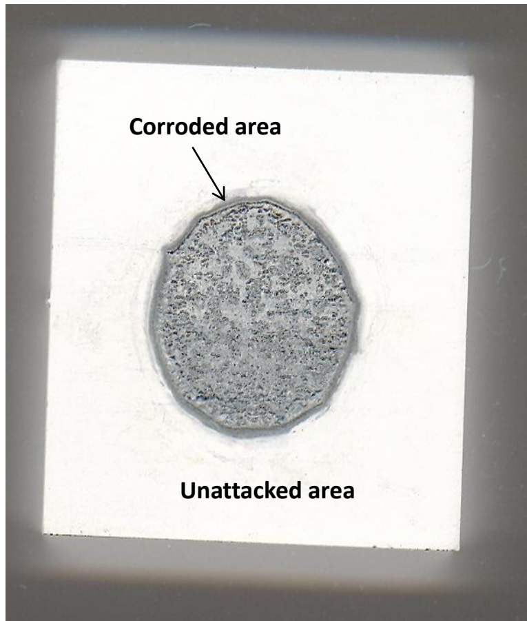
Fig. 4.152: Photograph of surface of crofer steel sample after corrosion testing for 24 h in 3.5% NaCl solution.
