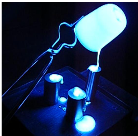
Fig. 3.2: Process of pouring the glass in steel mould at 1500 °C.
