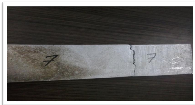
Figure 5.18 Broken sample after UTM Experimentation
