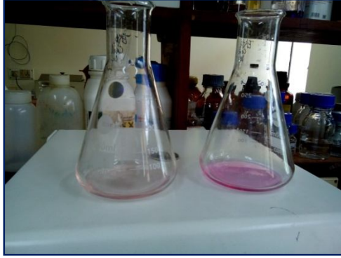
Figure 3.3 Development of pink color in the end point titration method of carbon dioxide estimation
