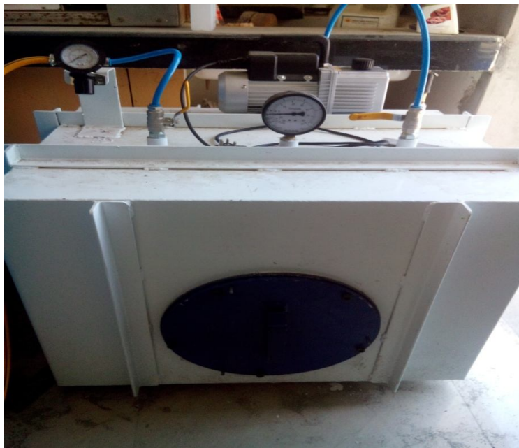
Figure 3.5 Carbonation curing chamber for curing cement mortar cubes.
