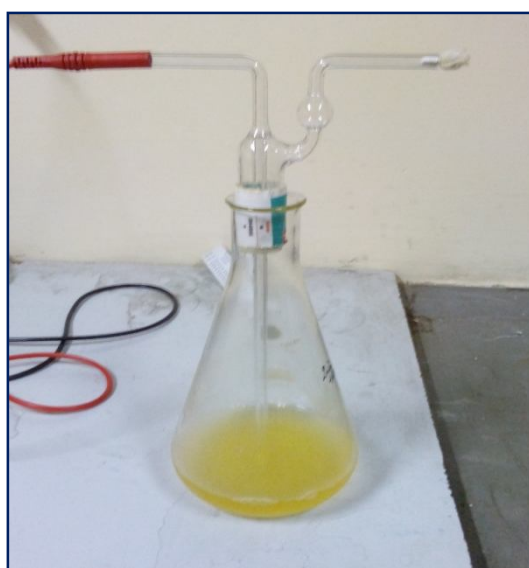
Figure 3.1 Apparatus used to flush carbon dioxide in the flasks.
